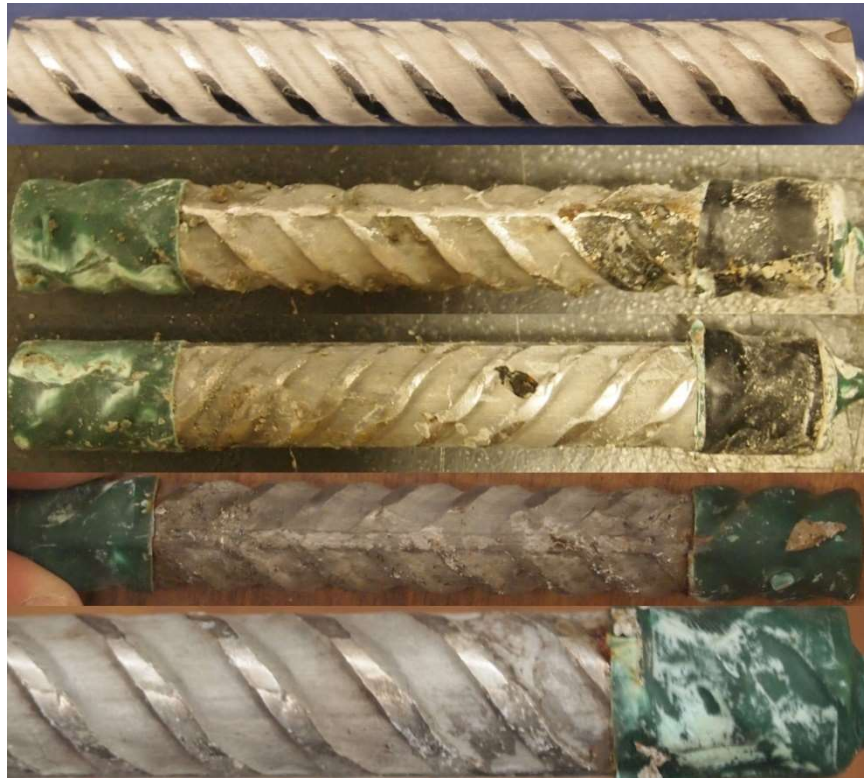
Figure C.49: 7.5-300 Batch – Corrosion Products on XM-28 AR 7.1. From top to bottom, a) original specimen, b) & c) corrosion products on the specimen upon removal from concrete, and d) & e) pitting corrosion identification on the pickled specimen. The slight staining at the top of the bar in a) is due to soldering flux.
