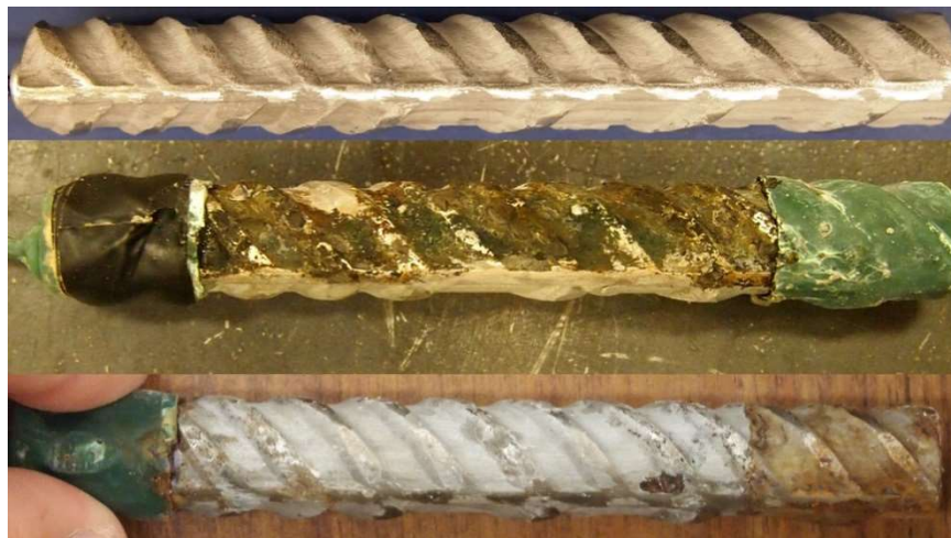
Figure C.2: RST 4-400 Batch – Corrosion Products on XM-28 AR 7.6. From top to bottom, a) original specimen, b) corrosion products on specimen upon removal from concrete, and c) pitting corrosion identification on a pickled specimen
