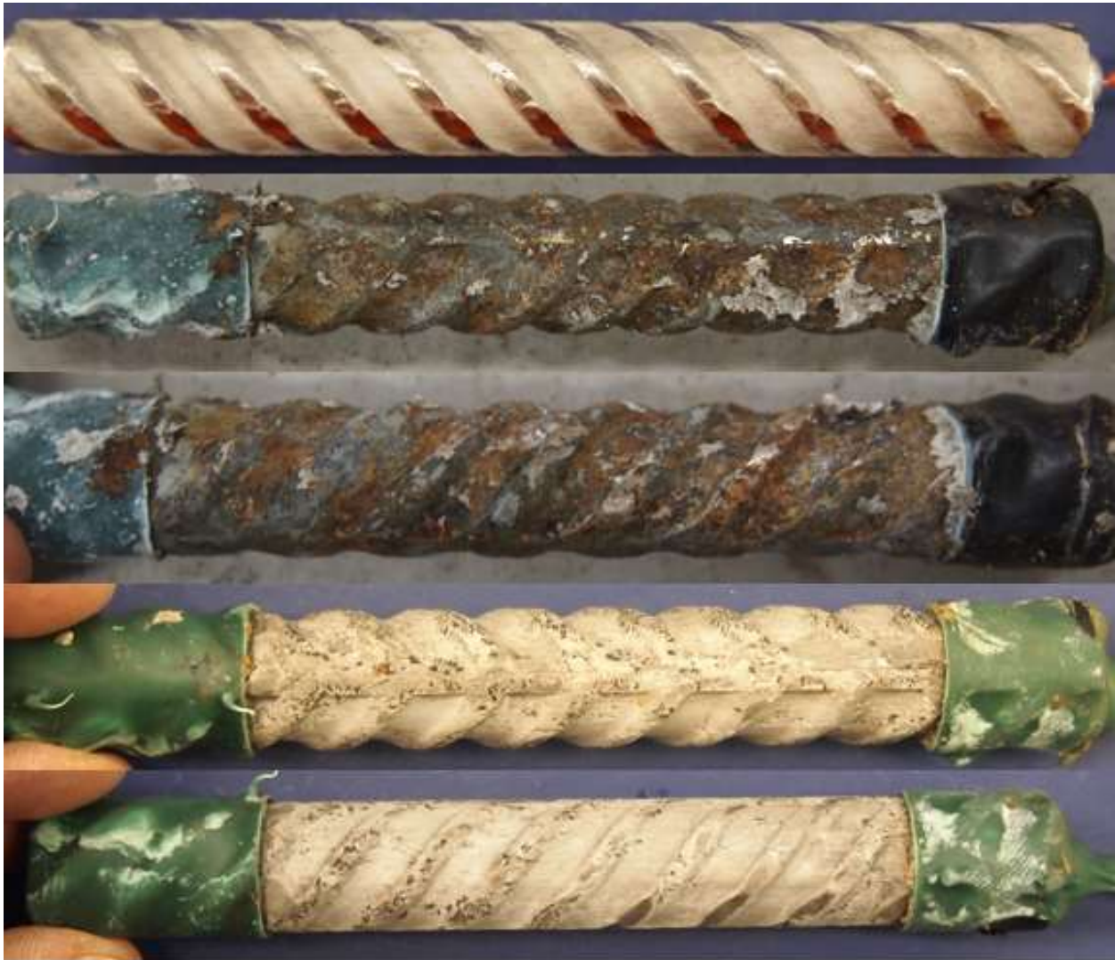
Figure 4.14: RST 7.5-400 Batch – Corrosion Products on XM-28 AR 8.1. From top to bottom, a) original specimen, b) & c) corrosion products on the specimen upon removal from concrete, and d) & e) pitting corrosion identification on the pickled specimen
