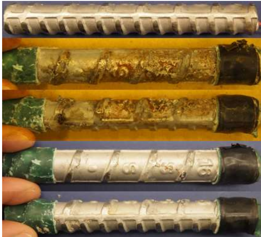
Figure C.74: 7.5-400 Batch – Corrosion Products on 2205 AR 7.6. From top to bottom, a) original specimen, b) & c) corrosion products on the specimen upon removal from concrete, and d) & e) pitting corrosion identification on the pickled specimen
