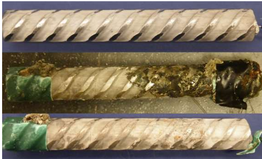
Figure C.8: 6-400 Batch – Corrosion Products on XM-28 AR 6.1. From top to bottom, a) original specimen, b) corrosion products on specimen upon removal from concrete, and c) pitting corrosion identification on the pickled specimen
