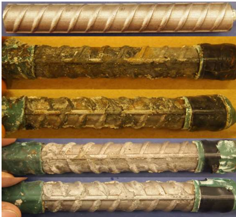
Figure C.59: 7.5-400 Batch – Corrosion Products on 2304 AR 7.2. From top to bottom, a) original specimen, b) & c) corrosion products on the specimen upon removal from concrete, and d) & e) pitting corrosion identification on the pickled specimen
