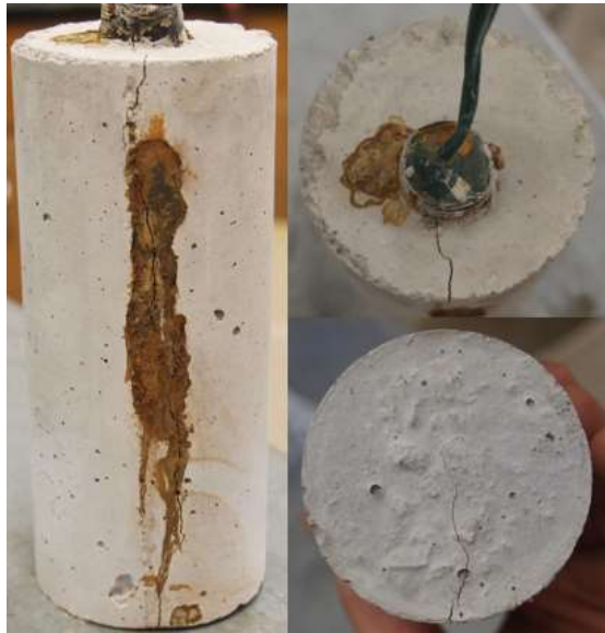
Figure C.77: RST 7.5-400 Batch – 2304 AR 7.6 Corrosion Products causing Cracking of Concrete Specimen
