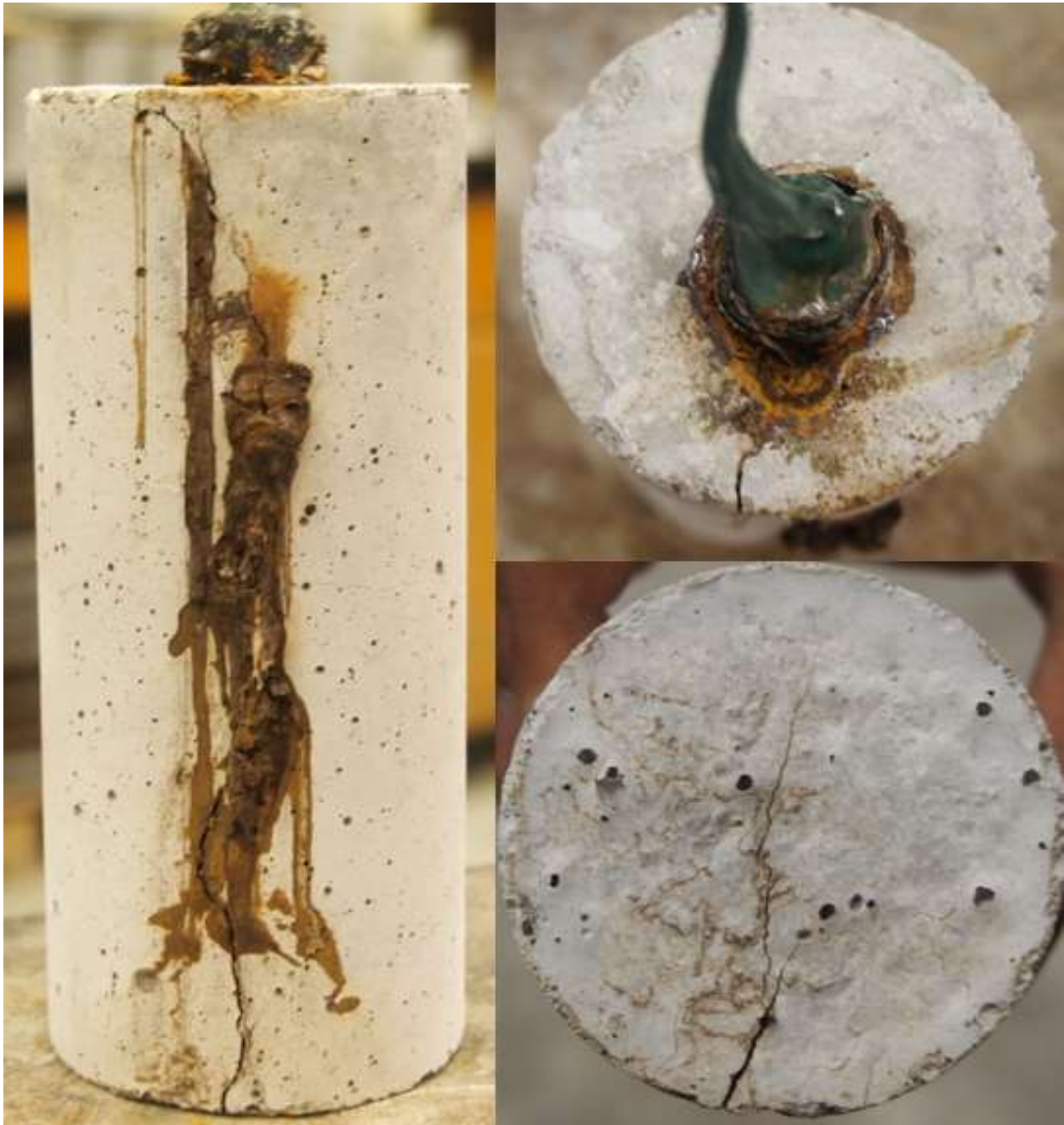
Figure 4.13: RST 7.5-400 Batch – XM-28 AR 8.1 Corrosion Products causing Cracking of Concrete Specimen
