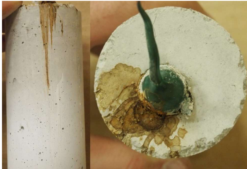
Figure C.20: RST 7.5-200 Batch – XM-28 AR 8.8 Corrosion Products causing Cracking of Concrete Specimen
