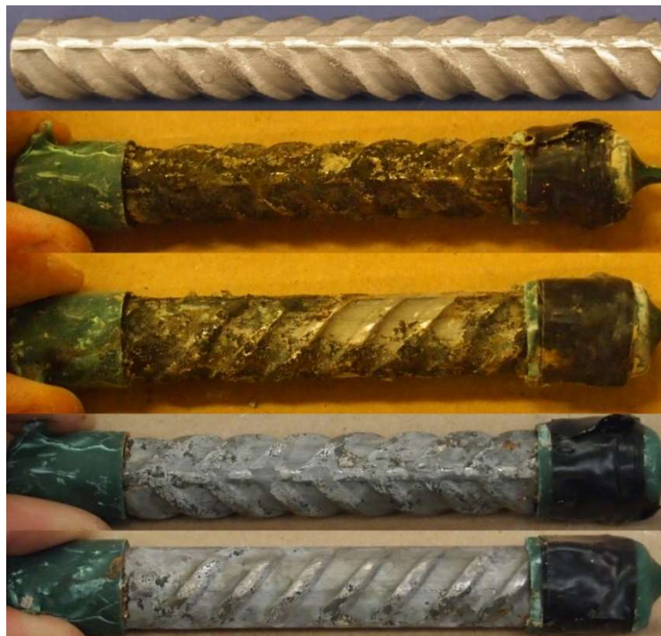
Figure C.32: 7.5-200 Batch – Corrosion Products on XM-28 AR 9.1. From top to bottom, a) original specimen, b) & c) corrosion products on the specimen upon removal from concrete, and d) & e) pitting corrosion identification on the pickled specimen
