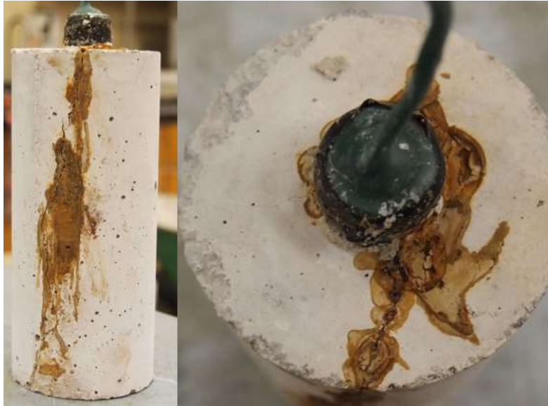
Figure C.75: RST 7.5-400 Batch – 2304 AR 7.5 Corrosion Products causing Cracking of Concrete Specimen
