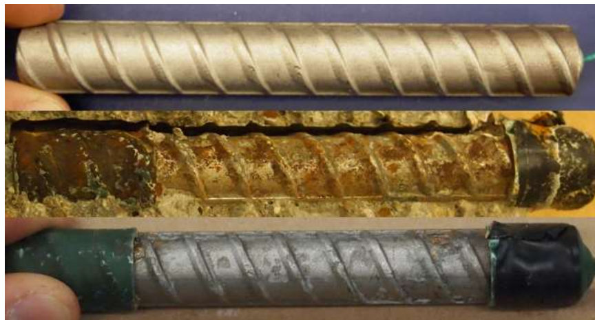
Figure C.25: 7.5-200 Batch – Corrosion Products on 2304 AR 7.9. From top to bottom, a) original specimen, b) corrosion products on the specimen upon removal from concrete, and c) pitting corrosion identification on the pickled specimen
