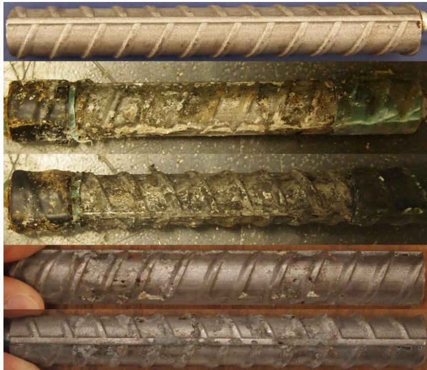
Figure C.40: 7.5-300 Batch – Corrosion Products on 2304 AR 5.7. From top to bottom, a) original specimen, b) & c) corrosion products on the specimen upon removal from concrete, and d) & e) pitting corrosion identification on the pickled specimen
