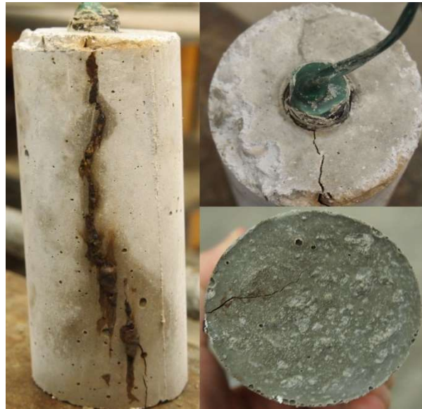
Figure C.45: RST 7.5-300 Batch – XM-28 AR 6.7 Corrosion Products Cracking the Concrete Specimen
