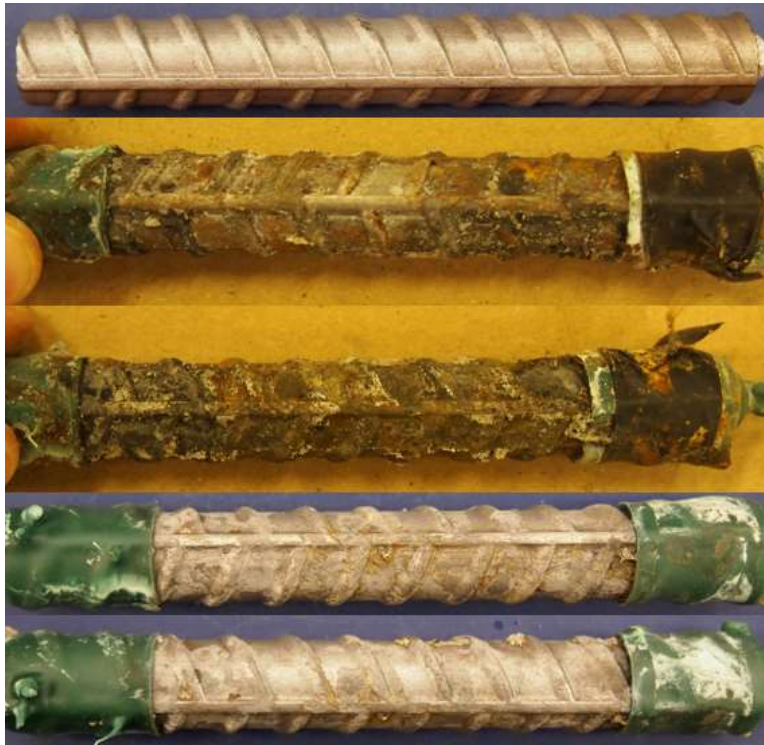
Figure C.57: 7.5-400 Batch – Corrosion Products on 2304 AR 7.1. From top to bottom, a) original specimen, b) & c) corrosion products on the specimen upon removal from concrete, and d) & e) pitting corrosion identification on the pickled specimen. The slight staining at the top of the bar in a) is due to soldering flux.
