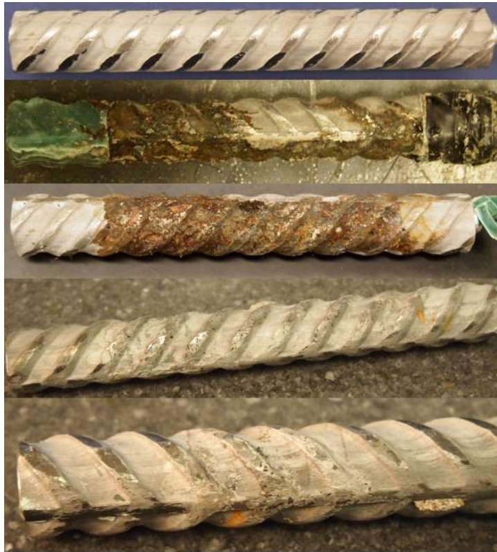
Figure C.16: 6-400 Batch – Corrosion Products on XM-28 AR 6.5. From top to bottom, a) original specimen, b) corrosion products on the specimen upon removal from concrete, c) oxidized corrosion products, and d) & e) pitting corrosion identification on the pickled specimen
