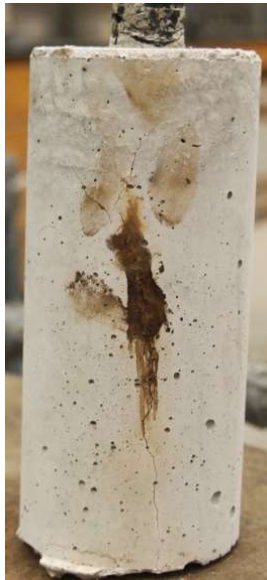
Figure C.15: RST 6-400 Batch – XM-28 AR 6.5 Corrosion Products causing Cracking of Concrete Specimen
