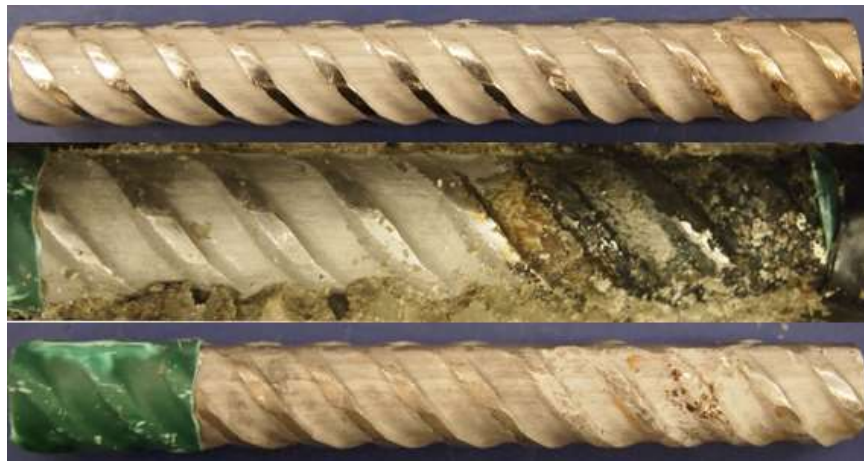
Figure C.6: RST 6-300 Batch – Corrosion Products on XM-28 AR 5.4. From top to bottom, a) original specimen, b) corrosion products on specimen upon removal from concrete, and c) pitting corrosion identification on the pickled specimen
