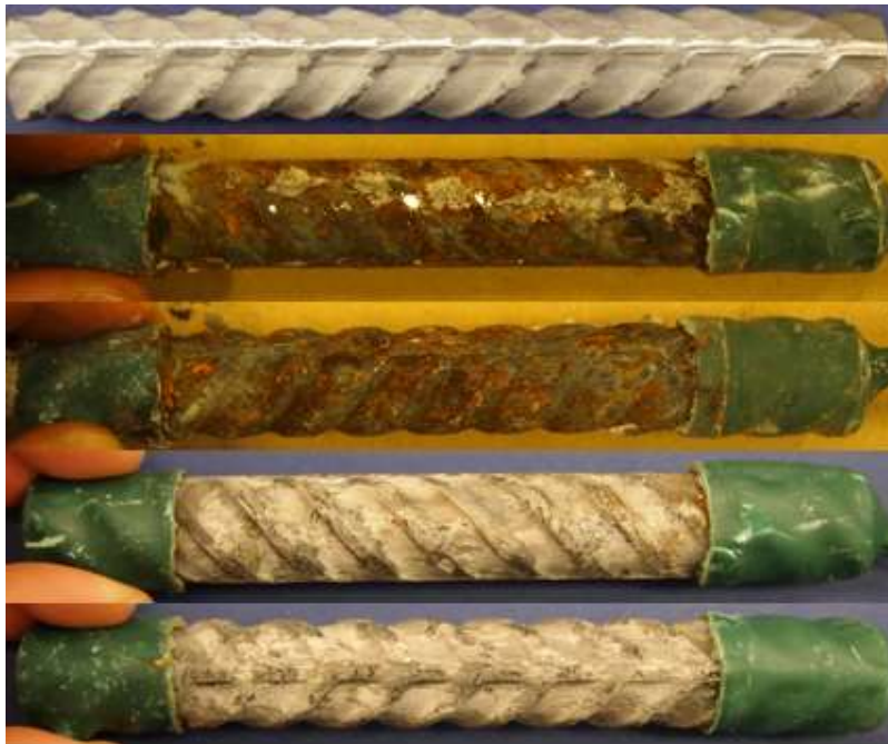
Figure C.82: 7.5-400 Batch – Corrosion Products on XM-28 AR 8.6. From top to bottom, a) original specimen, b) & c) corrosion products on the specimen upon removal from concrete, and d) & e) pitting corrosion identification on the pickled specimen. The slight staining at the top of the bar in a) is due to soldering flux.
