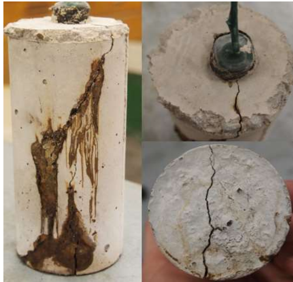
Figure C.79: RST 7.5-400 Batch – XM-28 AR 8.5 Corrosion Products causing Cracking of Concrete Specimen
