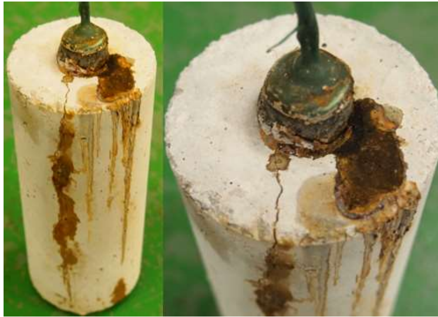
Figure C.68: RST 7.5-400 Batch – 2304 AR 7.4 Corrosion Products causing Cracking of Concrete Specimen
