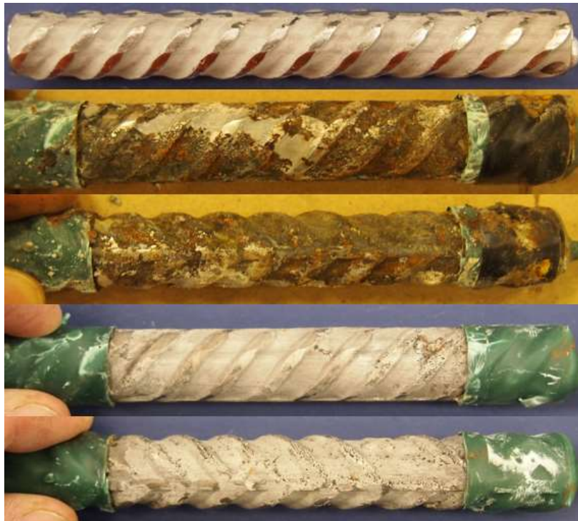
Figure C.63: 7.5-400 Batch – Corrosion Products on XM-28 AR 8.2. From top to bottom, a) original specimen, b) & c) corrosion products on the specimen upon removal from concrete, and d) & e) pitting corrosion identification on the pickled specimen
