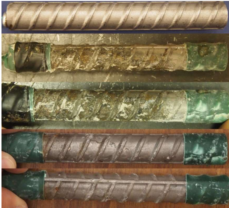
Figure C.55: 7.5-300 Batch – Corrosion Products on 2304 AR 6.4. From top to bottom, a) original specimen, b) & c) corrosion products on the specimen upon removal from concrete, and d) & e) pitting corrosion identification on the pickled specimen
