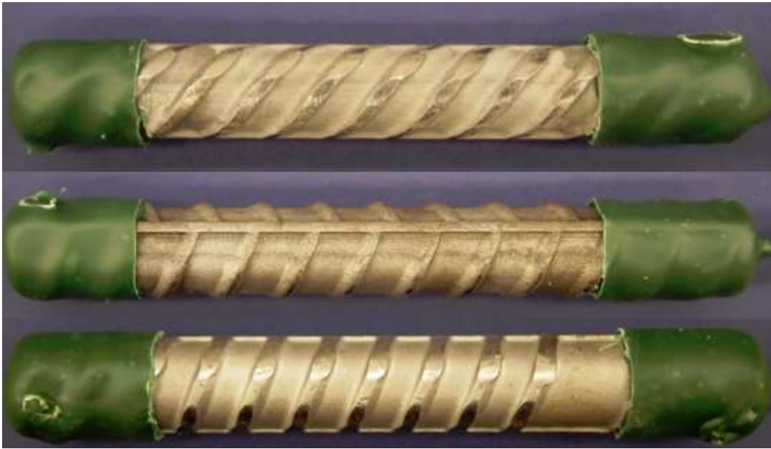
Figure 3.2: Rapid Screening Test Specimens with Lacquered Ends. From top to bottom, a) S24100 (XM-28), b) S32304, and c) S32205
