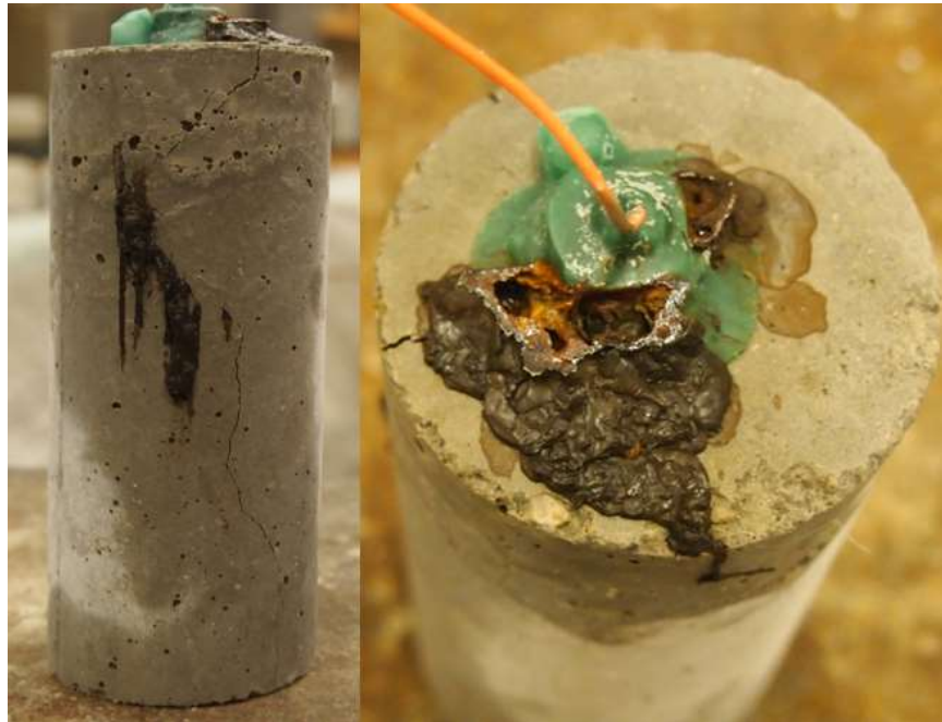
Figure C.9: RST 6-400 Batch – XM-28 AR 6.2 Corrosion Products causing Cracking of Concrete Specimen
