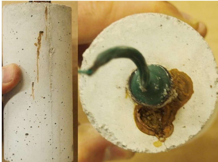
Figure C.24: RST 7.5-200 Batch – 2304 AR 7.9 Corrosion Products causing Cracking of Concrete Specimen
