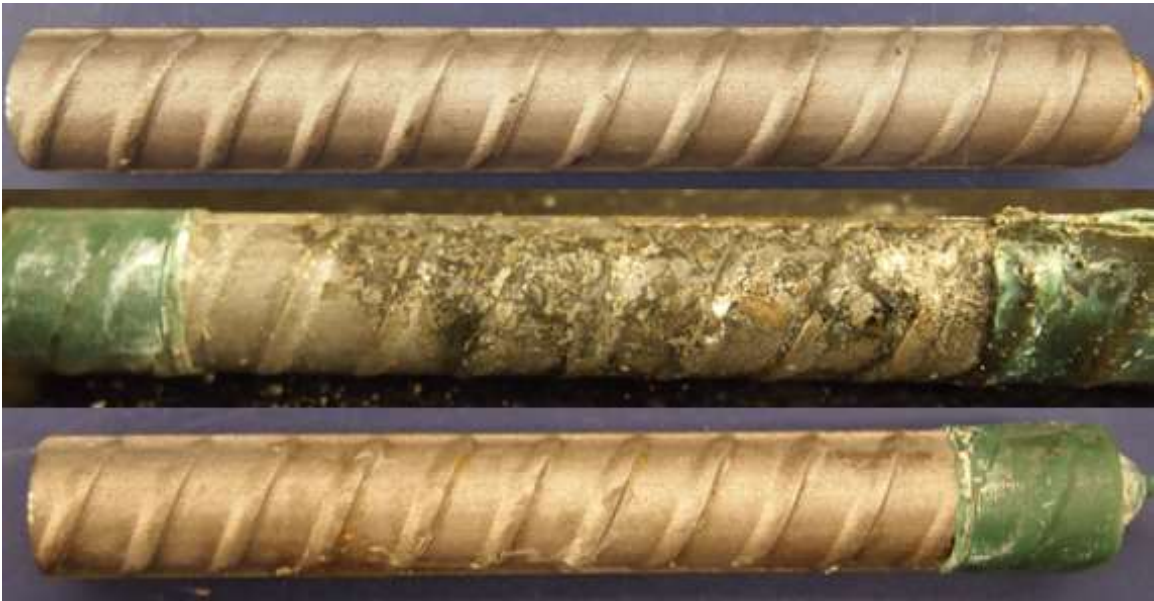
Figure 4.15: RST 6-300 Batch – Corrosion Products on 2304 AR 4.3. From top to bottom, a) original specimen, b) corrosion products on specimen upon removal from concrete, and c) pitting corrosion identification on the pickled specimen
