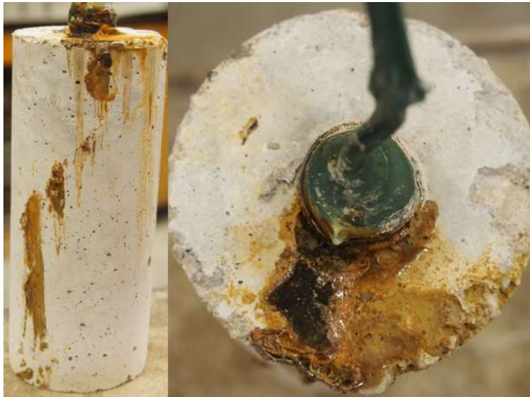
Figure C.58: RST 7.5-400 Batch – 2304 AR 7.2 Corrosion Products causing Cracking of Concrete Specimen
