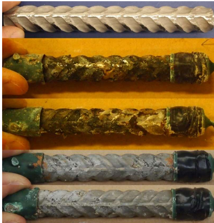
Figure C.34: 7.5-200 Batch – Corrosion Products on XM-28 AR 9.2. From top to bottom, a) original specimen, b) & c) corrosion products on the specimen upon removal from concrete, and d) & e) pitting corrosion identification on the pickled specimen
