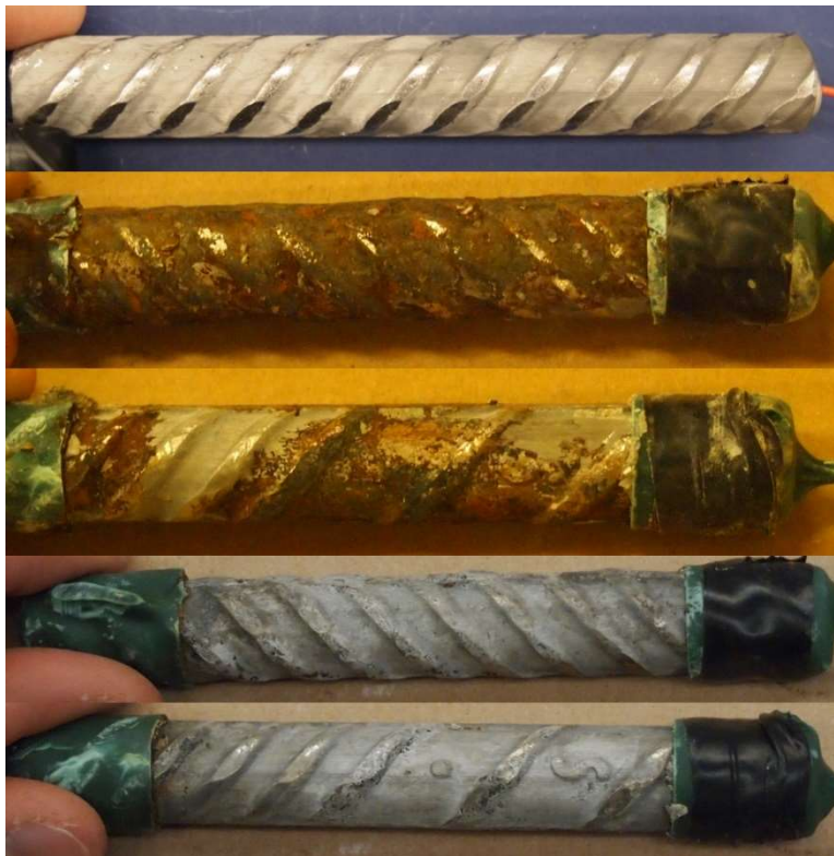
Figure C.19: 7.5-200 Batch – Corrosion Products on XM-28 AR 8.7. From top to bottom, a) original specimen, b) & c) corrosion products on the specimen upon removal from concrete, and d) & e) pitting corrosion identification on the pickled specimen
