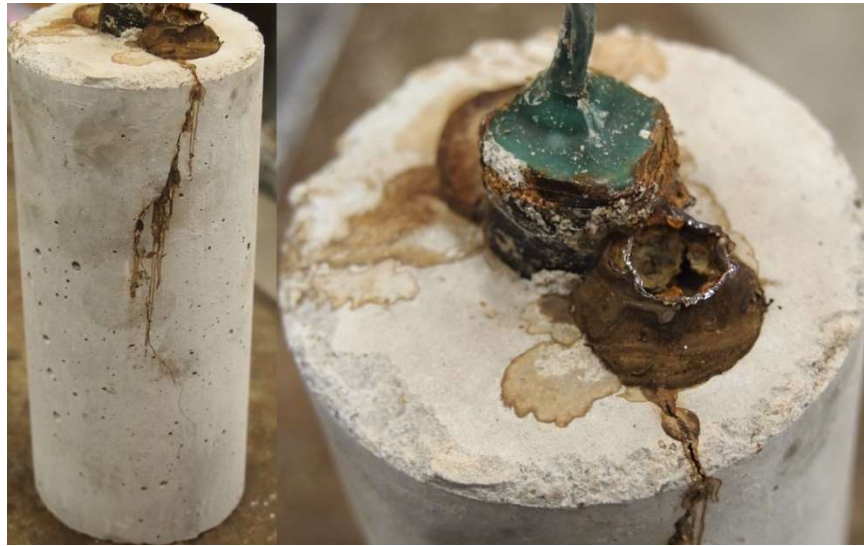
Figure C.47: RST 7.5-300 Batch – XM-28 AR 6.8 Corrosion Products Cracking the Concrete Specimen
