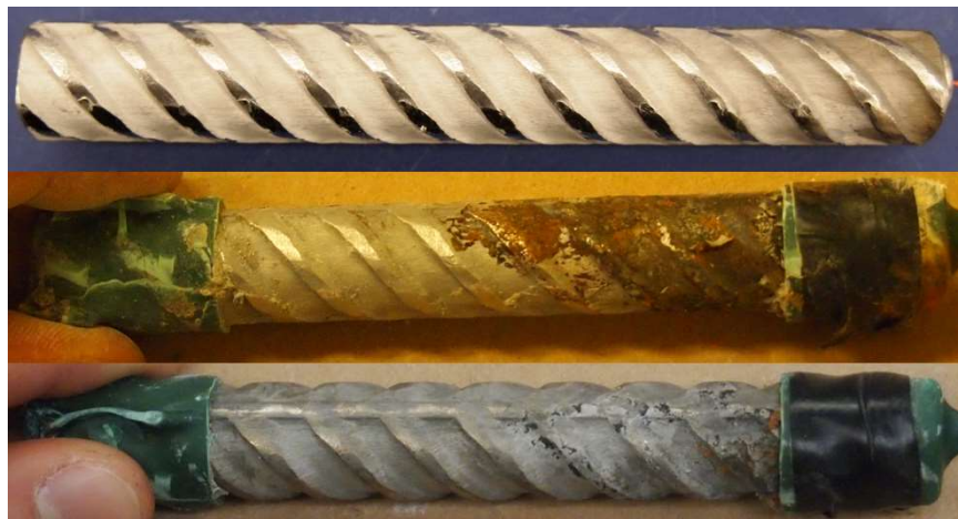
Figure C.21: 7.5-200 Batch – Corrosion Products on XM-28 AR 8.8. From top to bottom, a) original specimen, b) corrosion products on the specimen upon removal from concrete, and c) pitting corrosion identification on the pickled specimen
