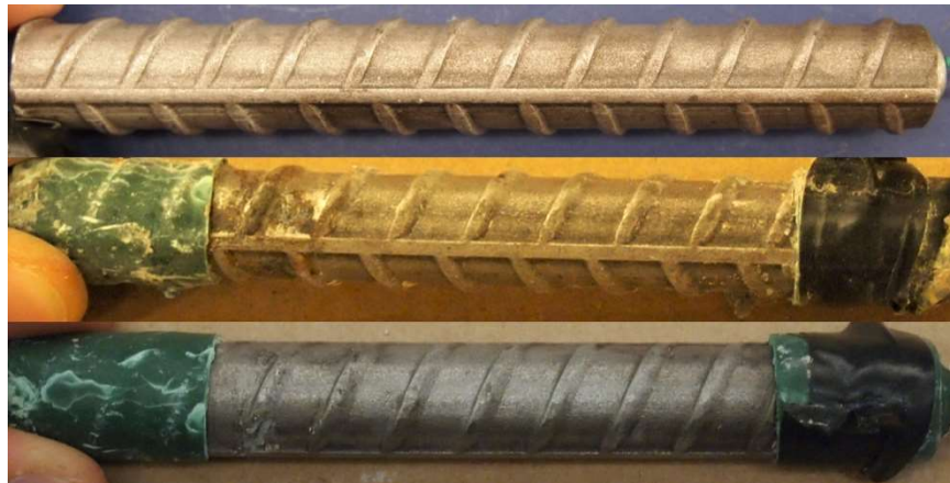
Figure C.23: 7.5-200 Batch – Corrosion Products on 2304 AR 7.8. From top to bottom, a) original specimen, b) corrosion products on the specimen upon removal from concrete, and c) pitting corrosion identification on the pickled specimen
