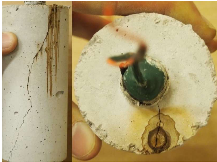
Figure C.18: RST 7.5-200 Batch – XM-28AR 8.7 Corrosion Products causing Cracking of Concrete Specimen
