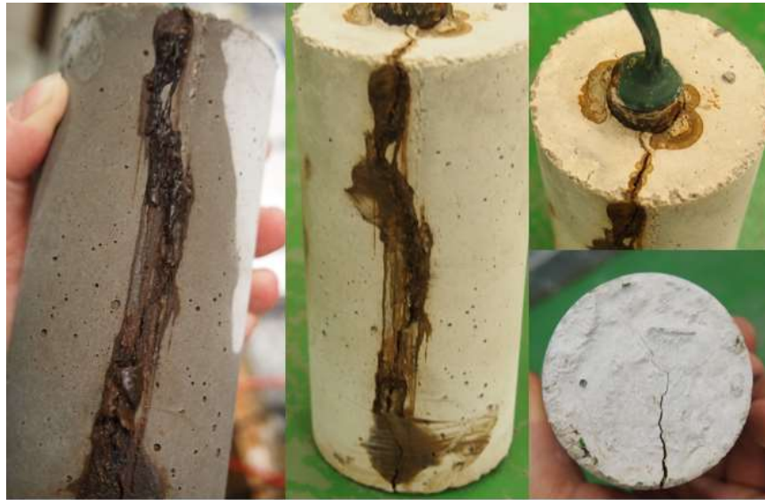
Figure C.72: RST 7.5-400 Batch – XM-28 AR 8.4 Corrosion Products causing Cracking of Concrete Specimen
