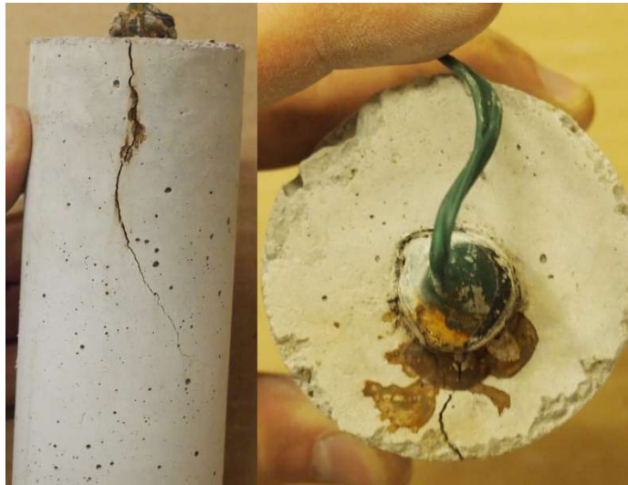
Figure C.27: RST 7.5-200 Batch – XM-28 AR 8.9 Corrosion Products causing Cracking of Concrete Specimen
