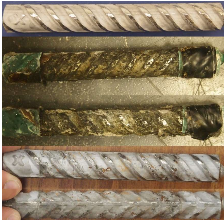
Figure C.46: 7.5-300 Batch – Corrosion Products on XM-28 AR 6.7. From top to bottom, a) original specimen, b) & c) corrosion products on the specimen upon removal from concrete, and d) & e) pitting corrosion identification on the pickled specimen
