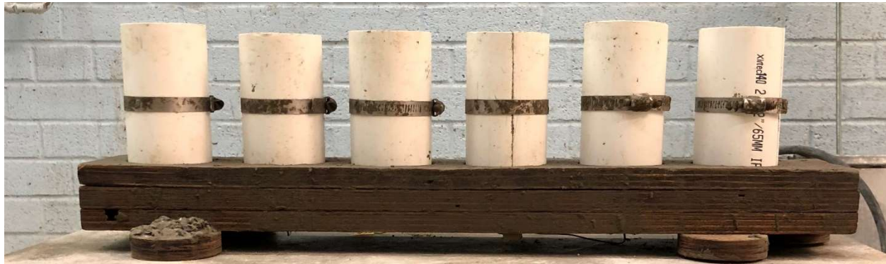
Figure 3.3: Concrete Moulds for the Rapid Screening Test Specimens
