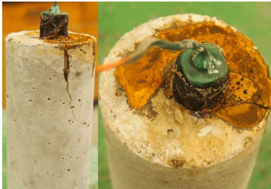
Figure C.12: RST 6-400 Batch – XM-28 AR 6.4 Corrosion Products causing Cracking of Concrete Specimen
