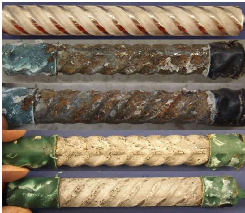
Figure C.61: 7.5-400 Batch – Corrosion Products on XM-28 AR 8.1. From top to bottom, a) original specimen, b) & c) corrosion products on the specimen upon removal from concrete, and d) & e) pitting corrosion identification on the pickled specimen
