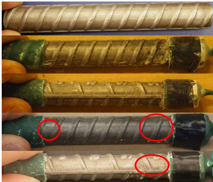
Figure C.36: 7.5-200 Batch – Corrosion Products on 2304 AR 8.2. From top to bottom, a) original specimen, b) & c) corrosion products on the specimen upon removal from concrete, and d) & e) pitting corrosion identification on the pickled specimen
