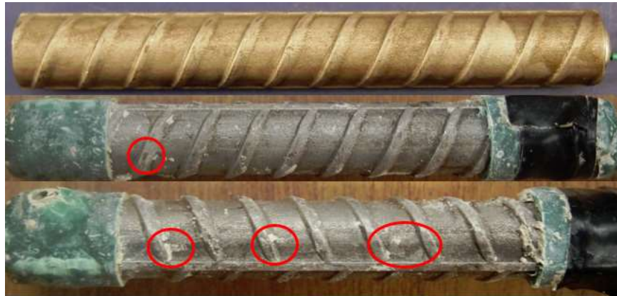
Figure C.35: 7.5-200 Batch – Corrosion Products on 2304 AR 8.1. From top to bottom, a) original specimen, and b) & c) corrosion products on the specimen upon removal from concrete. Identification of pitting corrosion was observed 4 months after the autopsy. The slight staining at the top of the bar in a) is due to soldering flux.
