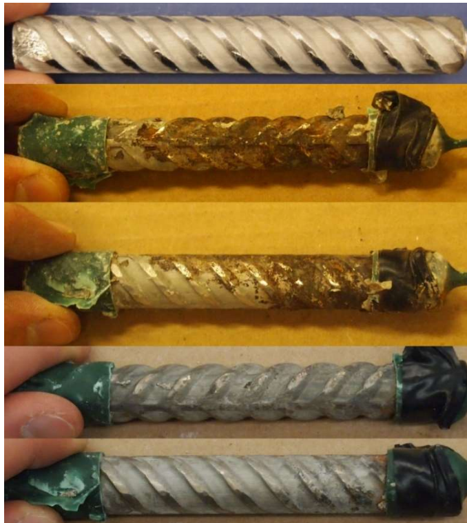
Figure C.28: 7.5-200 Batch – Corrosion Products on XM-28 AR 8.9. From top to bottom, a) original specimen, b) & c) corrosion products on the specimen upon removal from concrete, and d) & e) pitting corrosion identification on the pickled specimen. The slight staining at the top of the bar in a) is due to soldering flux.
