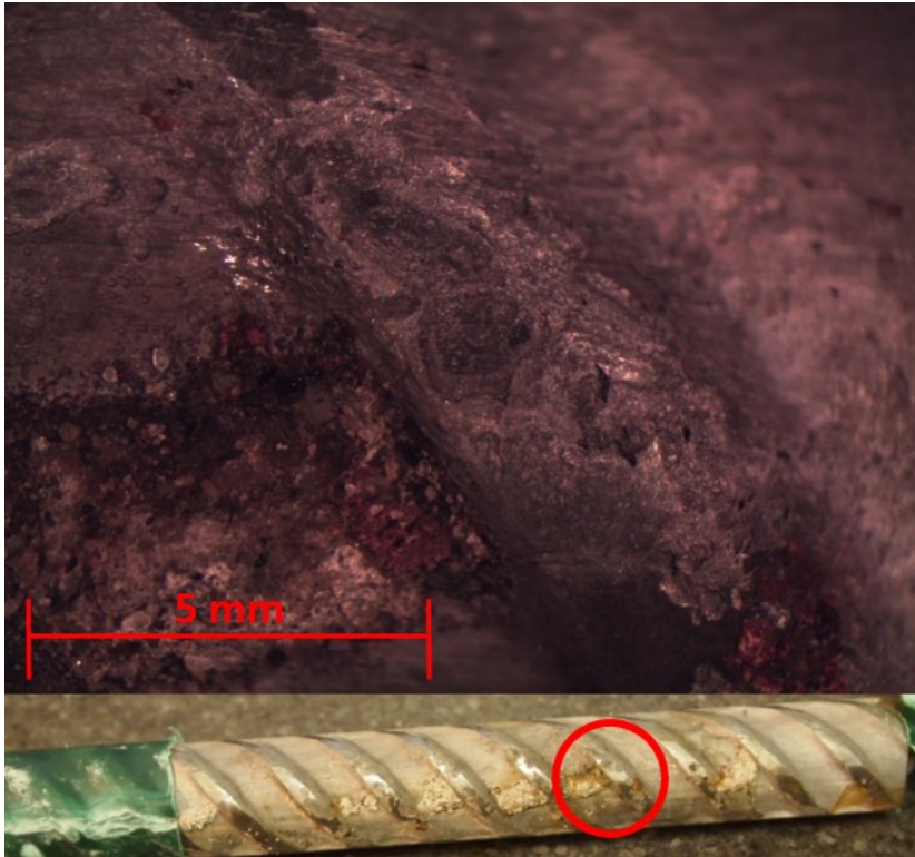
Figure D.7: RST Batch 6-400 Photomicrographs: a) pickled XM-28 AR 6.3 and b) pickled XM-28 AR 6.4. Staining from corrosion products observed underneath the lacquer on XM-28 AR 6.4
