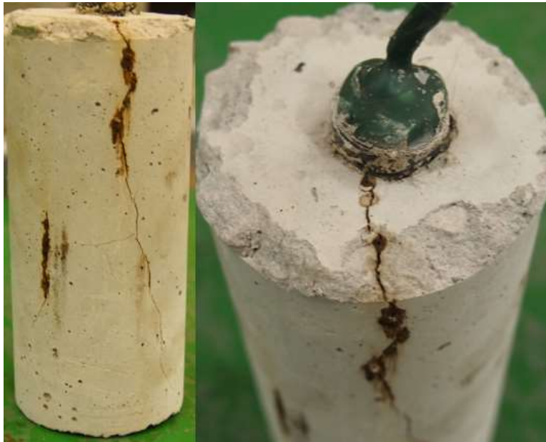
Figure C.70: RST 7.5-400 Batch – XM-28 AR 8.3 Corrosion Products causing Cracking of Concrete Specimen
