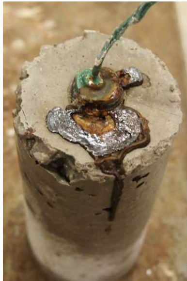
Figure C.7: RST 6-400 Batch – XM-28 AR 6.1 Corrosion Products Observed on Concrete Specimen
