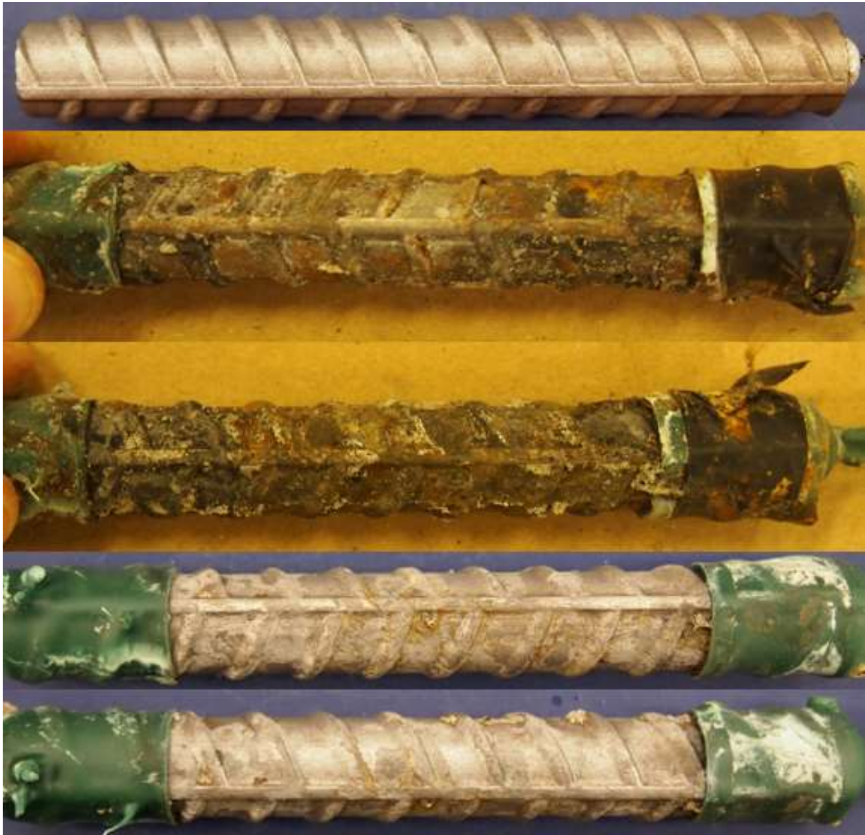
Figure 4.17: RST 7.5-400 Batch – Corrosion Products on 2304 AR 7.1. From top to bottom, a) original specimen, b) & c) corrosion products on the specimen upon removal from concrete, and d) & e) pitting corrosion identification on the pickled specimen
