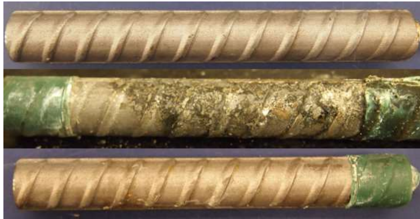
Figure C.5: RST 6-300 Batch – Corrosion Products on 2304 AR 4.3. From top to bottom, a) original specimen, b) corrosion products on specimen upon removal from concrete, and c) pitting corrosion identification on the pickled specimen
