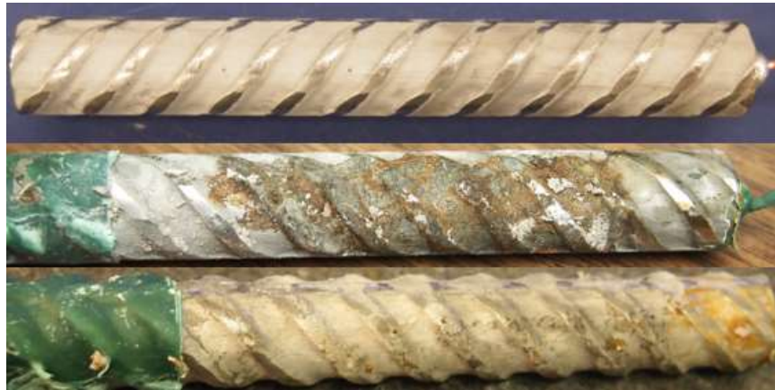
Figure C.13: 6-400 Batch – Corrosion Products on XM-28 AR 6.4. From top to bottom, a) original specimen, b) corrosion products on specimen upon removal from concrete, and c) pitting corrosion identification on the pickled specimen
