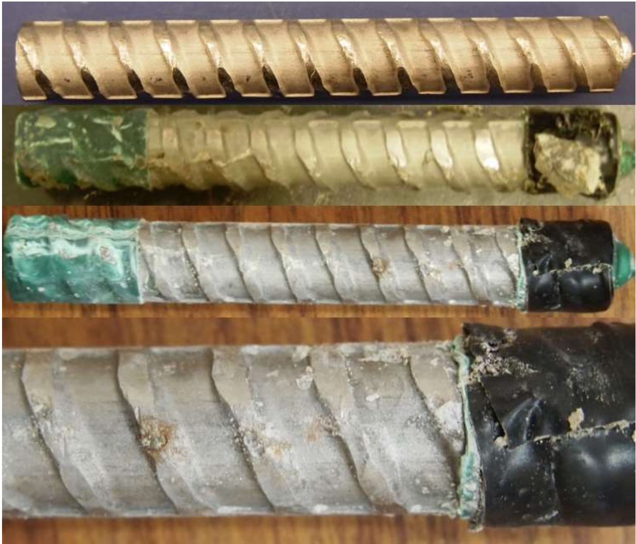
Figure 4.18: 6-400 Batch – Evidence of Pitting Corrosion on 2205 AR 5.5. From top to bottom, a) original specimen, b) corrosion products on specimen upon removal from concrete, and c) & d) pitting corrosion identification on the pickled specimen. Identification of pitting corrosion was observed 1 week after autopsy.
