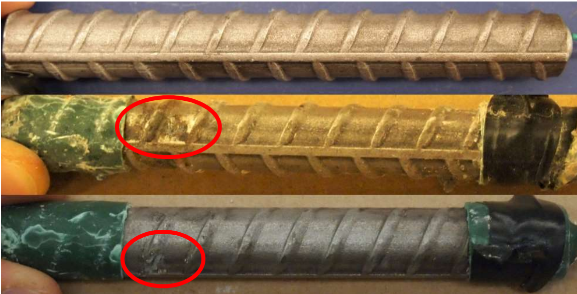
Figure 6.5: 7.5-200 Batch – Corrosion Products on 2304 AR 7.8. From top to bottom, a) original specimen, b) corrosion products on the specimen upon removal from concrete, and c) pitting corrosion identification on the pickled specimen
