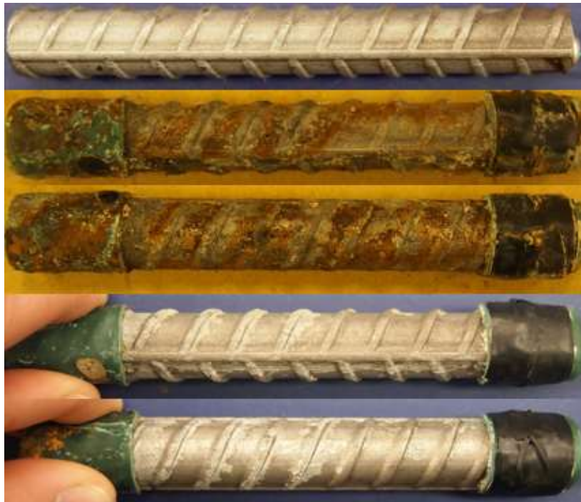
Figure C.78: 7.5-400 Batch – Corrosion Products on 2304 AR 7.6. From top to bottom, a) original specimen, b) & c) corrosion products on the specimen upon removal from concrete, and d) & e) pitting corrosion identification on the pickled specimen
