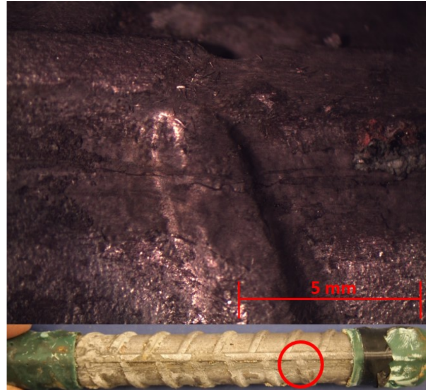
Figure D.26: RST Batch 7.5-400 Photomicrographs: a) pickled 2304 AR 7.1 and b) pickled 2304 AR 7.2
