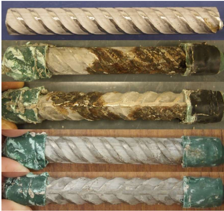
Figure C.3: RST 4-400 Batch – Corrosion Products on XM-28 AR 7.7. From top to bottom, a) original specimen, b) corrosion products on specimen upon removal from concrete, and c) pitting corrosion identification on a pickled specimen
