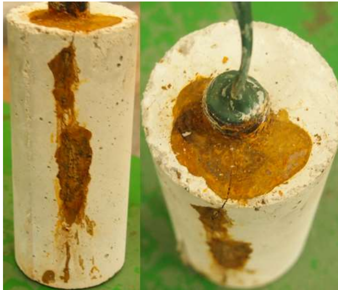
Figure C.66: RST 7.5-400 Batch – 2304 AR 7.3 Corrosion Products causing Cracking of Concrete Specimen
