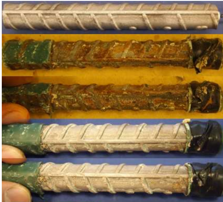
Figure C.69: 7.5-400 Batch – Corrosion Products on 2304 AR 7.4. From top to bottom, a) original specimen, b) & c) corrosion products on the specimen upon removal from concrete, and d) & e) pitting corrosion identification on the pickled specimen
