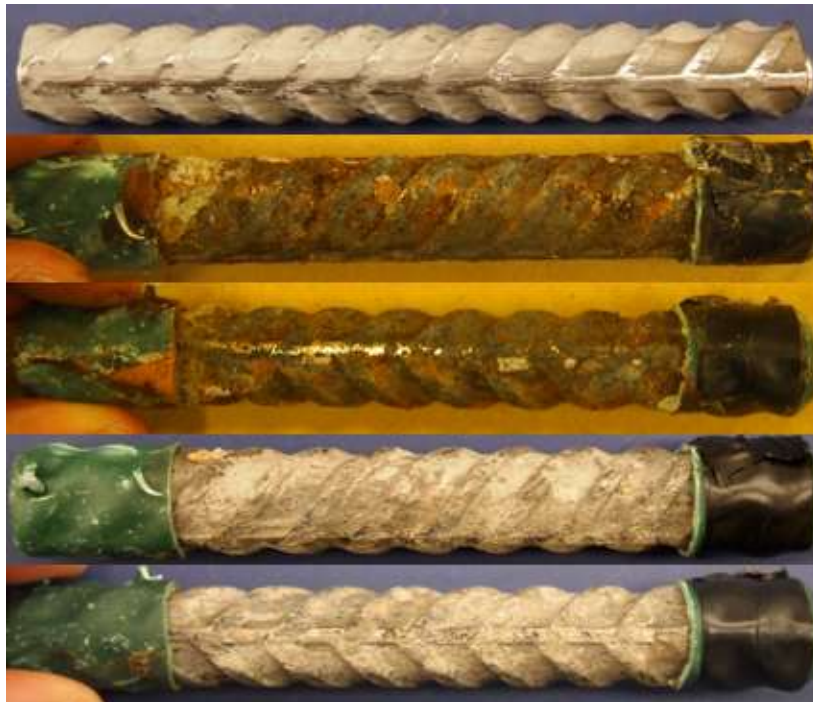
Figure C.80: 7.5-400 Batch – Corrosion Products on XM-28 AR 8.5. From top to bottom, a) original specimen, b) & c) corrosion products on the specimen upon removal from concrete, and d) & e) pitting corrosion identification on the pickled specimen. The slight staining at the top of the bar in a) is due to soldering flux.
