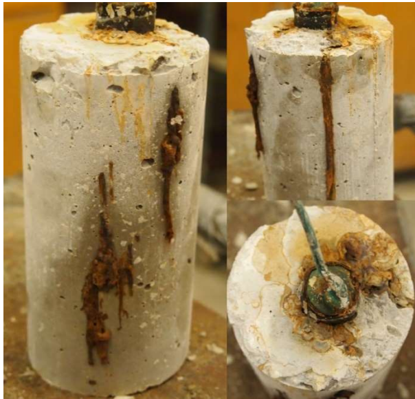
Figure C.39: RST 7.5-300 Batch – 2304 AR 5.7 Corrosion Products Leaking through Concrete Specimen
