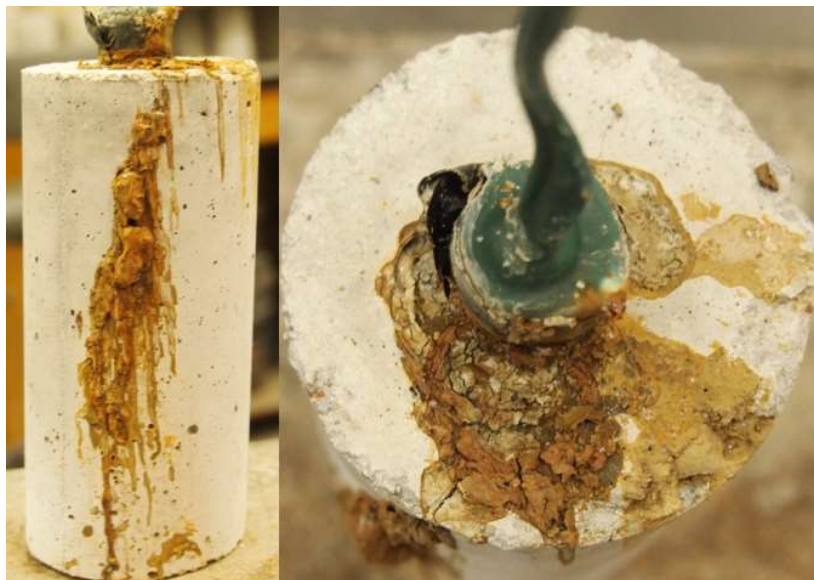
Figure C.56: RST 7.5-400 Batch – 2304 AR 7.1 Corrosion Products causing Cracking of Concrete Specimen
