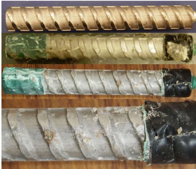
Figure C.17: 6-400 Batch – Evidence of Pitting Corrosion on 2205 AR 5.5. From top to bottom, a) original specimen, b) corrosion products on specimen upon removal from concrete, and c) & d) pitting corrosion identification on the pickled specimen. Identification of pitting corrosion was observed 1 week after the autopsy.
