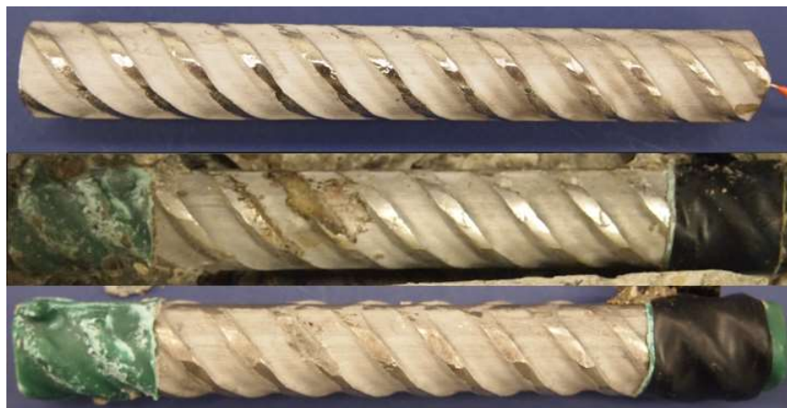
Figure C.4: RST 6-200 Batch – Corrosion Products on XM-28 AR 5.2. From top to bottom, a) original specimen, b) corrosion products on specimen upon removal from concrete, and c) pitting corrosion identification on a pickled specimen
