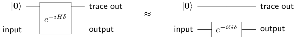
Figure 4.3: The Local Hamiltonian Approximation lemma. The first register is M -dimensional, the second register contains n qubits, and the approximation is within O(\delta^2) (independent of M and n ).
