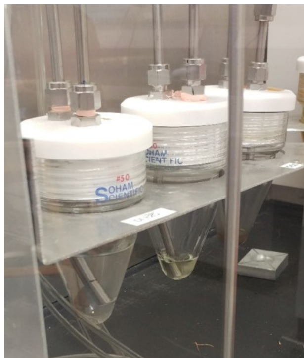
Figure 2.3: Bubblers used to hold the precursors and generate precursor gases in the AP-SALD
