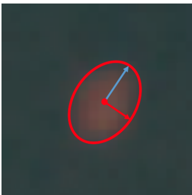
Figure 4.4: Visualization of a skewed projection point as approximated by an Elliptical 2D Gaussian PSF. Directions of the arrow represent eigenvectors of the Gaussian covariance, and their lengths are proportional to their eigenvalues. The minimum eigenvalue (length of the red arrow) is used as the depth feature, since it is less affected by the distortion.
