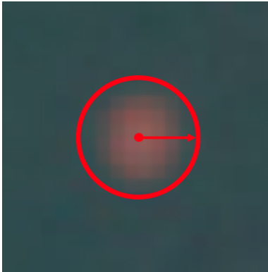
Figure 4.2: Visualization of a projected point pattern as approximated by a circularly-symmetric 2D Gaussian PSF. The red arrow illustrates the standard deviation of the Gaussian distribution as the depth feature to characterize the spread of blurring.
