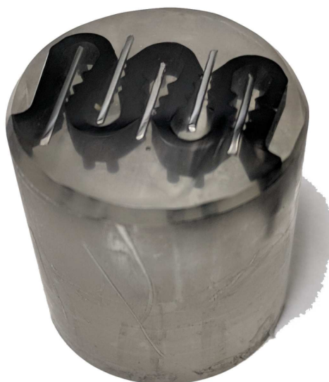
Figure 3.4: Optical imaging sample showing five NiTi wires with visible cross-sections ready for optical imaging after mounting and polishing.
