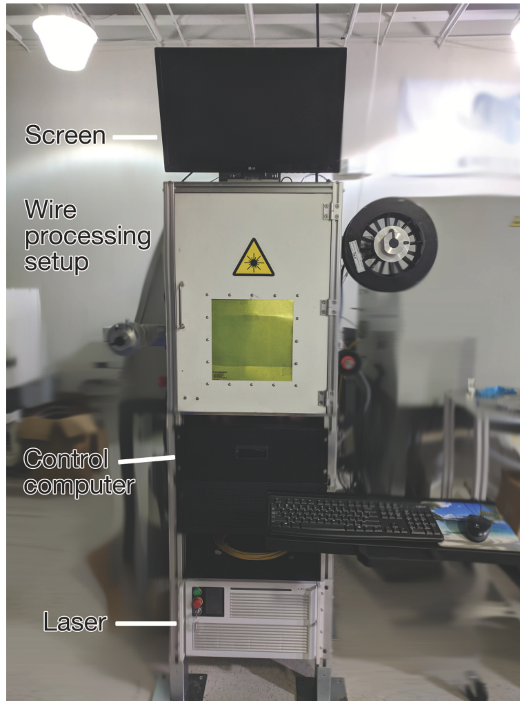
Figure 3.5: System used for producing laser processed NiTi wires.
