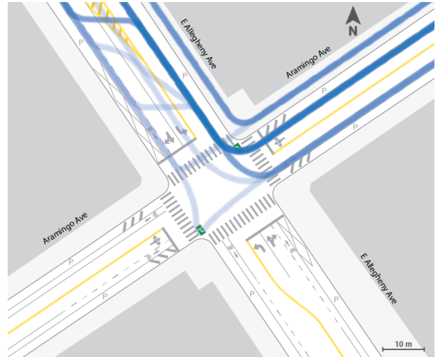
Figure 2: Intersection 3 'After' Desire Lines of Southbound Left-turning Bicycles Arriving on Green and Red Signal Phases
