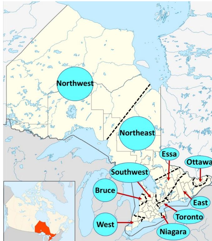
Figure 5.1: An overview of the boundaries separating the 10 different power zones in Ontario
