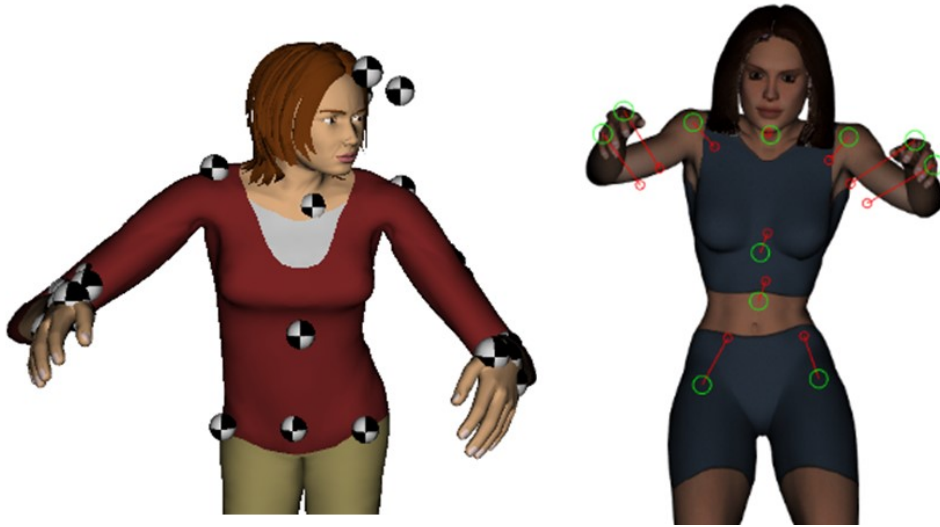
Figure 35. Joint position data from the lab-based model mapped onto anthropometrically scaled avatars in Jack (left) and Santos (right). In Santos, the green circles show the avatar joint centers of rotation and the red circles are the joint centers of rotation of the lab-based skeletal model, red lines show the mapping errors
