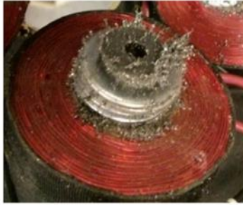
Figure 3. 3: Residual magnetism shown with particles sticking to the coil core.
