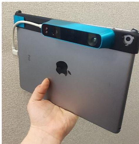
Figure 27. Structure IO, structured light scanner used for experiment mounted on an iPad
