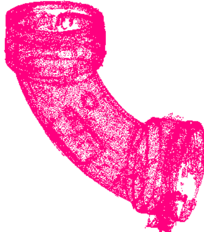
Figure 18. Point cloud of the elbow obtained with the FARO Arm scanner
