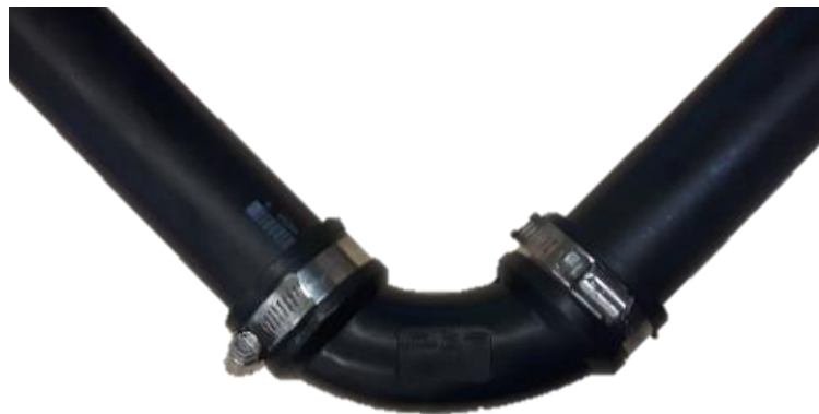
Figure 7. Flexible elbow coupling used to simulate socket welds
