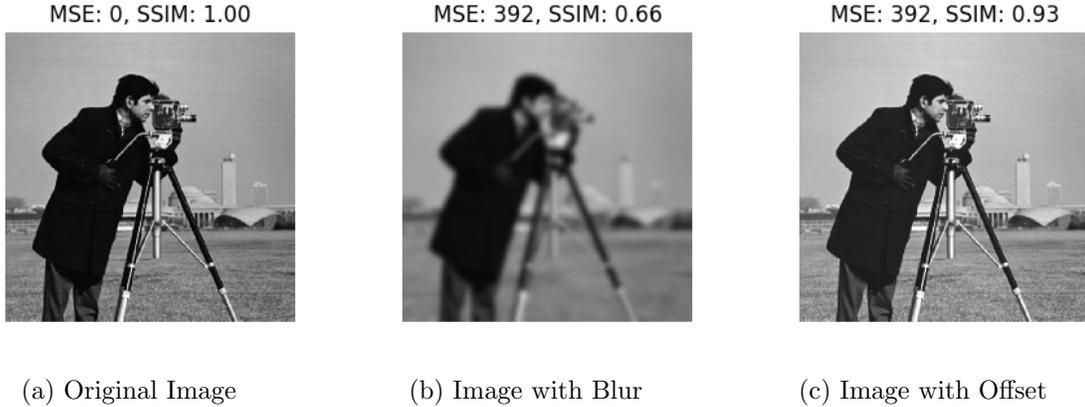
Figure 2.3: This figure compares MSE and SSIM in their ability to measure human visual perceptual differences between images. Two separate transforms are applied to the left most image (a): a Gaussian blur (b), and a global offset (c). Notice that the two transformed images have the same MSE but different SSIM. Comparatively, (c) is perceptually closer to the original image than (b). This is not reflected in MSE but is reflected in SSIM.
