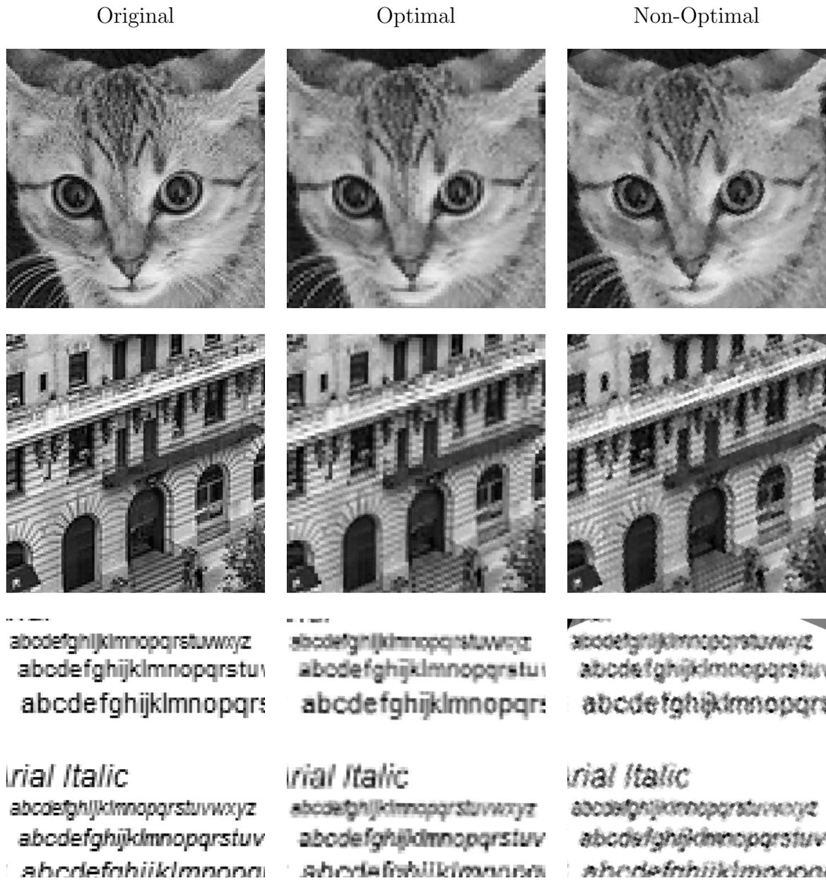
Figure 5.4: A comparison between an original image, a two projector system at the optimal configuration, and a two projector configuration at a non-optimal configuration. Both configurations have a PLR of  $\sqrt{2}$ . The non-optimal configuration has one projector rotated 22.5 degrees clockwise and the other projector rotated 22.5 degrees counter-clockwise. Notice that the sub-pixels in the non-optimal images do not resemble squares.
