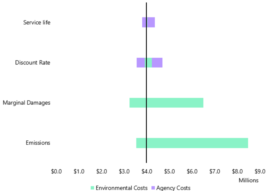
Figure 7.2 Uncertainty in total lifecycle cost of preferred design alternative (M2 CIR) ($2018 CAD)
