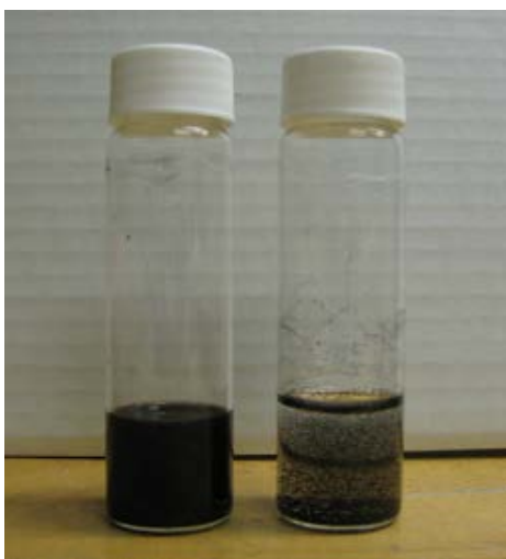
Figure 4-2 Picture of suspension of purified (left bottle) and unpurified (right bottle) SWCNTs in DI water
