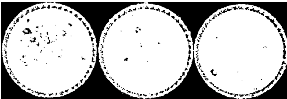
Figure 98. Representative figure showing the border region defects from Chapter 4. From left-to-right are samples one, two, and three, which correspond to 250 W power; 60 \mu\text{m} grid distance; and 60, 70, and 80 \mu\text{s} exposure time, respectively.
