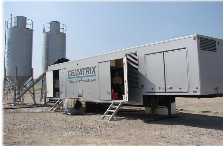
Figure 2-3: “Dry” Mix Equipment (Dolton et al., 2016)
