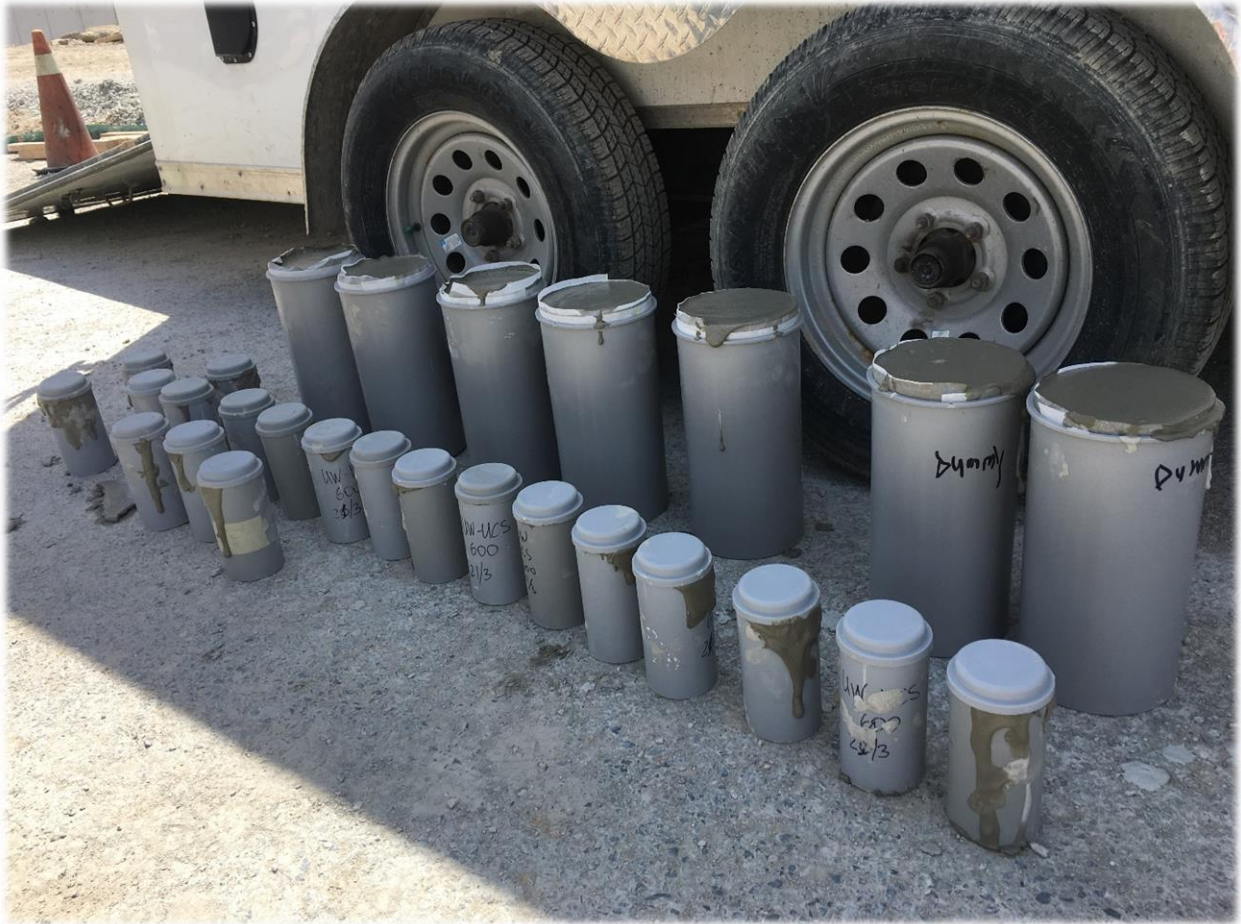
Figure 5-3: Samples, Collected on Site. 75*150 mm Molds for UCS test. 150*300 mm Molds for Modulus of Elasticity and Poisson's Ratio Tests
