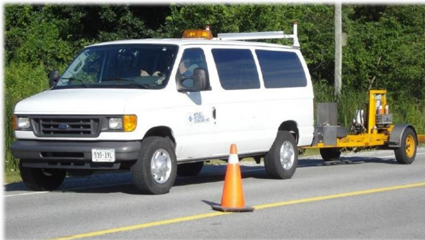
Figure 3-9: FWD Truck and Trailer (Griffiths and Popik, 2013)
