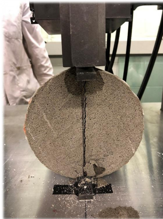
Figure 2-6: Splitting Tensile Strength Test Setup
