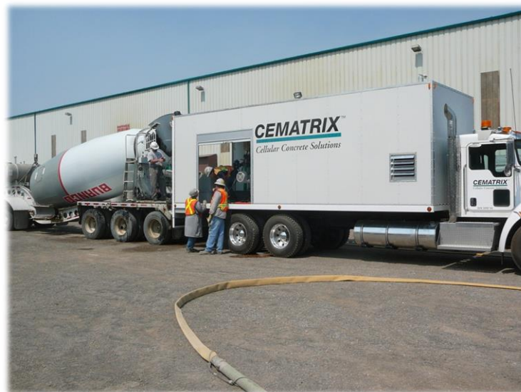
Figure 2-2: "Wet" Mix Equipment (Dolton et al., 2016)
