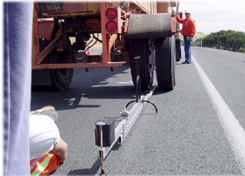
Figure 3-25: Benkelman Beam Deflection Testing
