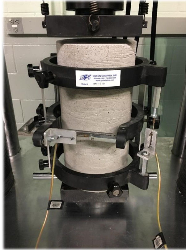
Figure 5-8: Modulus of Elasticity and Poisson's Ratio Test Setup
