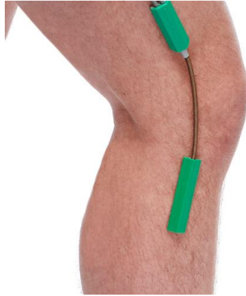
Figure 5.1: An example of the electrogoniometers from Biometrics, Ltd. that were used in the experiments [4]
