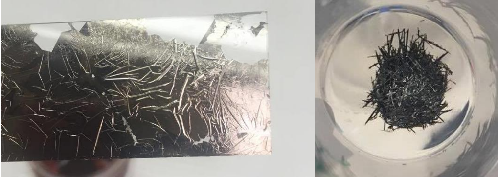
Figure 3-2 The sputtered structures (left) during the dissolving process for the photoresist layer, and (right) the free-standing structures after being removed from their substrate
