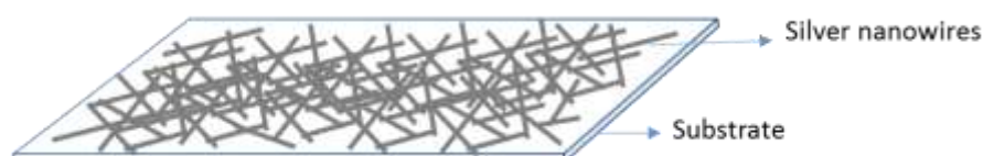
Figure 6: Schematic representation of a metallic NW network deposited randomly.
