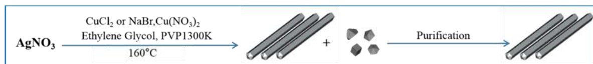
Figure 15: Scheme of the synthesis of ultra-long silver nanowires adopted. [108]
