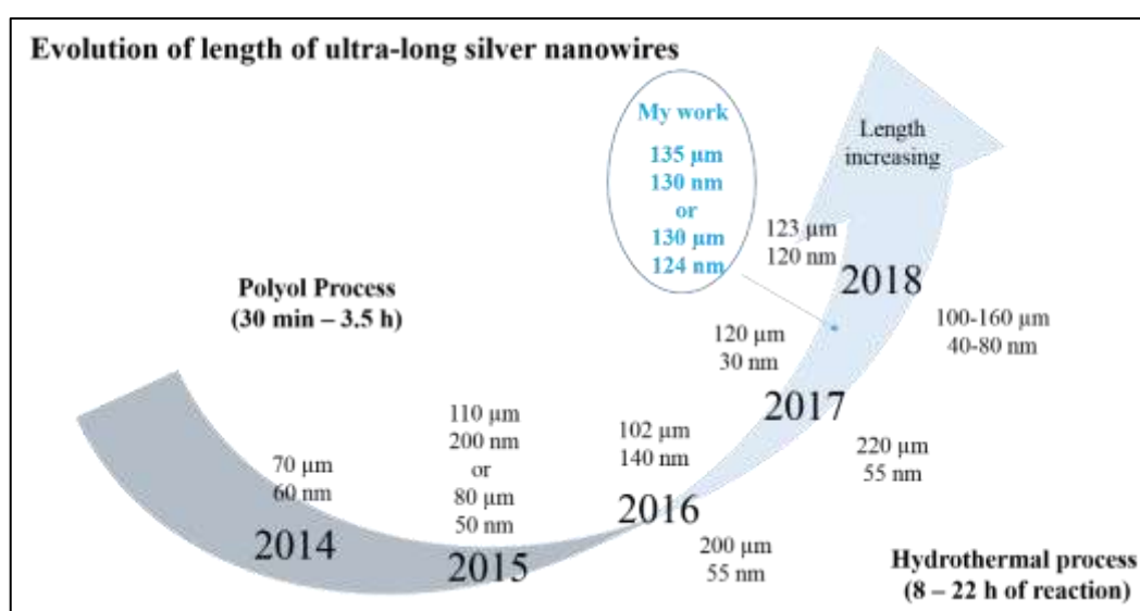
Figure A: Evolution of the length of the ultra-long silver nanowires published in the literature from 2014 to 2018. [65,86,87,89,90,108,111,112]
