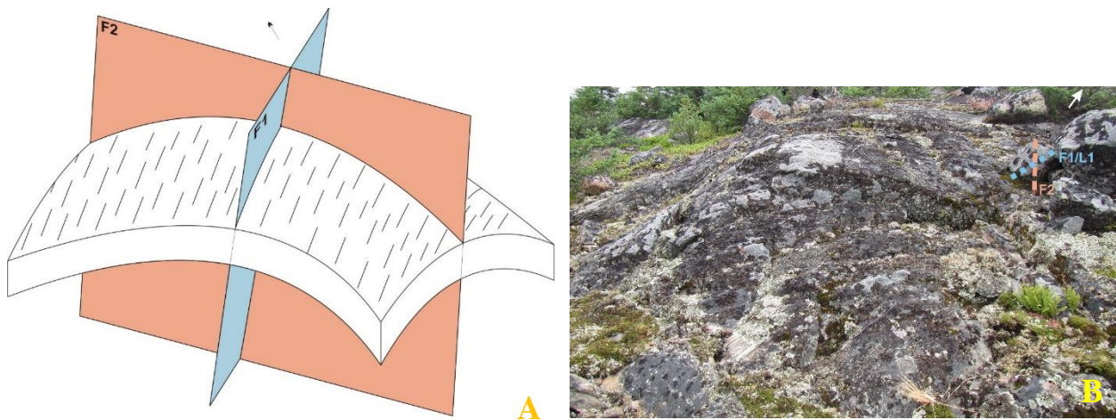
Figure 4-47. (A) Diagram showing a F1 fold refolded by a F2 fold, producing a canoe fold with a porpoising F2 fold hinge. L1 lineations are observed to trend parallel to the F1 fold hinge. (B) Outcrop photo of the fold. Heavy lichen cover and weathering obscure the majority of the fabrics.
