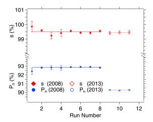
FIG. 9. (Color online) The neutron polarization (circles) and spin-flipper efficiency (diamonds) measured in 2008 (solid) and 2013 (open) determined using the asymmetry method. The uncertainties shown are purely statistical. Fits of the data are shown as solid lines for 2008 and dotted lines for 2013. Points with larger uncertainties were taken when the cell had lower polarization.
