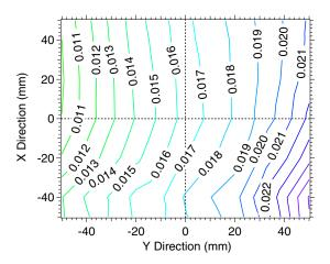
FIG. 8. (Color online) The difference between the maximum magnetic field in mT and the magnetic field  $B_z$  in the region of the target cell's center (0,0) measured using a fluxgate magnetometer. Contour lines show a  $7 \times 10^{-4}~{\rm cm}^{-1}$  field gradient.
