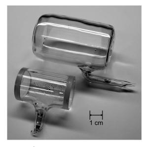
FIG. 4. Two <sup>3</sup>He cells. The larger of the two cells, called Skylight, was used in the polarimetry measurements. The smaller flat-window cell called Pistachio was used as a target cell. Rubidium deposits can be seen as dark spots along the walls of the cell.
