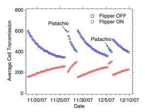
FIG. 7. (Color online) The average cell transmissions  $I^{\uparrow}$  (blue squares) and  $I^{\downarrow}$  (red circles) as measured by the C4 detector for a subset of the data that includes five cell transfers. The data taken with the cell Pistachio are marked. The statistical uncertainties are smaller than the points.
