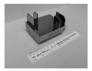
FIG. 3. The skew symmetric interferometer made by Cliff Holmes and others at the University of Missouri-Columbia machine shop (on loan from Dr. Samuel A. Werner).
