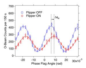
FIG. 5. (Color online) Typical interferograms generated by a off-on-on-off spin-flipper sequence is shown where the spin flipper is off (blue squares) and on (red circles). Each point was counted for 150 s. The lower intensity for the "Flipper ON" interferogram is attributable to stronger absorption in that case. The uncertainties shown are purely statistical. Lines are fits of the data using Eq. (20).
