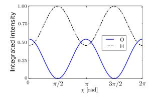
FIG. 7. The intensity of the O and H beams as a function of the phase between the two NI paths  $\chi$ . The simulation is done for N = 100 planes in each blade where the unitary operator of a single node is  $U_{j,0,0,\pi/4}$ .
