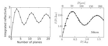
FIG. 4. The left figure is the integrated reflectivity at the exit of a single crystal based on the QI model with a node unitary operator  $U_{j,0,0,\theta=\pi/8}$ . The right figure is the measured integrated reflectivity of Bragg scattering in the Laue diffraction; see Fig. 1 of Ref. [24]. Copyright permission from Elsevier. In comparison a Si thickness of 50  $\mu$ m corresponds to three planes in the QI model.
