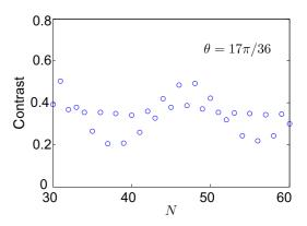
FIG. 8. The contrast of the H beam for a three-blade neutron interferometer as a function of the number of planes in each blade N. The unitary operator for each node is  $U_{j,0,0,17\pi/36}$ . To calculate the contrast, the phase difference between the two paths is varied over a full cycle. The maximum and minimum are then extracted to get the contrast using Eq. (40).
