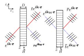
FIG. 1. Bragg diffraction from a crystal in the Laue geometry. In the Laue geometry the diffracted beam is on a different surface of the crystal relative to the incident beam. The two possible inputs to the crystal lead to different transmission and reflection coefficients for the waves exiting the crystal.
