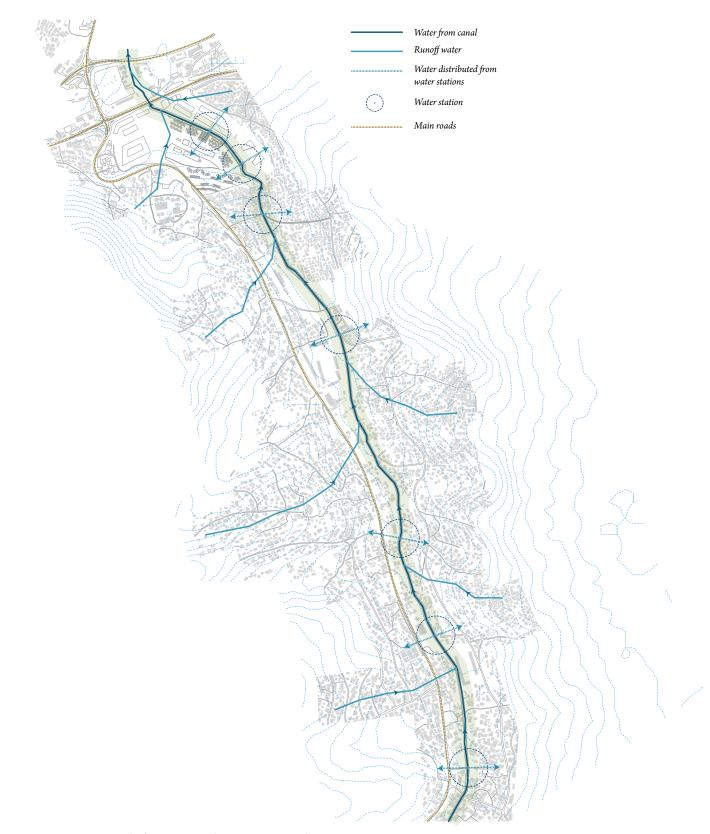
Figure 5.13: Network of water stations along Kimisagara canal
