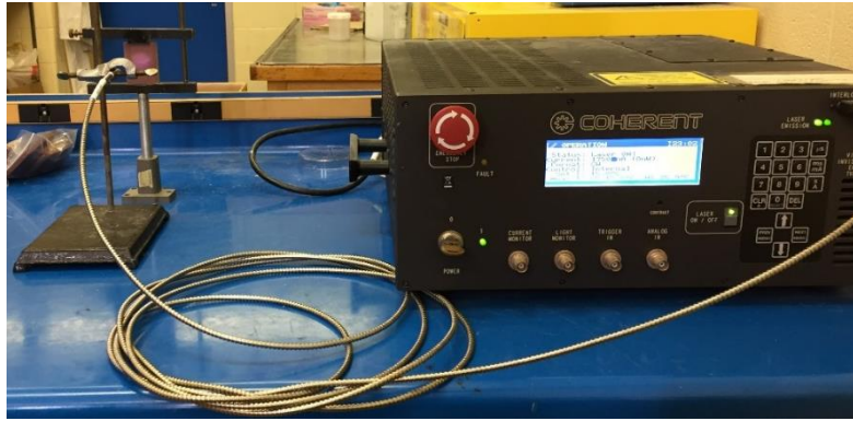
Figure 2.5 The experimental setup of laser erosion resistance measurement.
