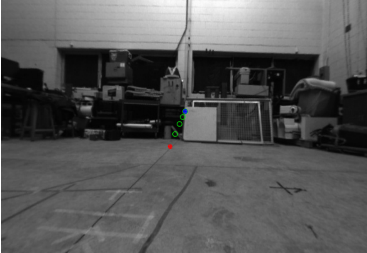
Figure 5.2: The epipole positions plotted on the key-frame image during an optimization process for a straight line motion. RED shows the epipole position due to noisy prior due to integration of IMU measurements at the start of the optimization. GREEN shows intermediate epipole positions during the optimization. BLUE is the final epipole position. Since the trajectory is straight, the epipole’s image on the key-frame image should be at the center of the image, which is where the initial noisy pose prior is driven to, as a result of optimization.
