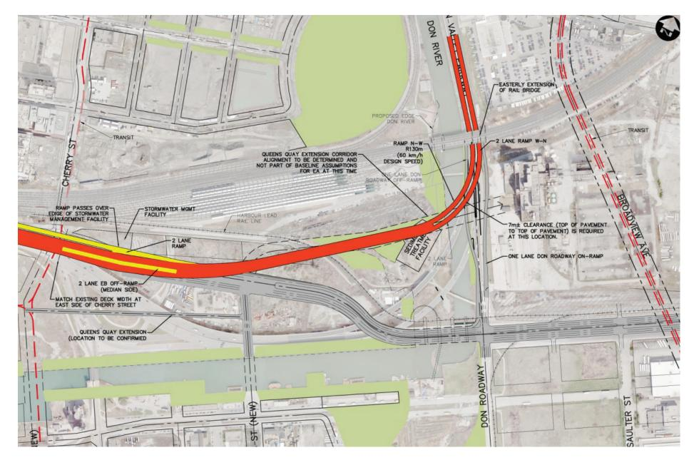
3.11 Hybrid Option Of Gardiner - Final Decision. The final decision is the hybrid option, which will create a boulevard at the east end by demolishing the existing ramp, and re-decking a portion of the highway by shifting it north while maintaining the number of lanes.
