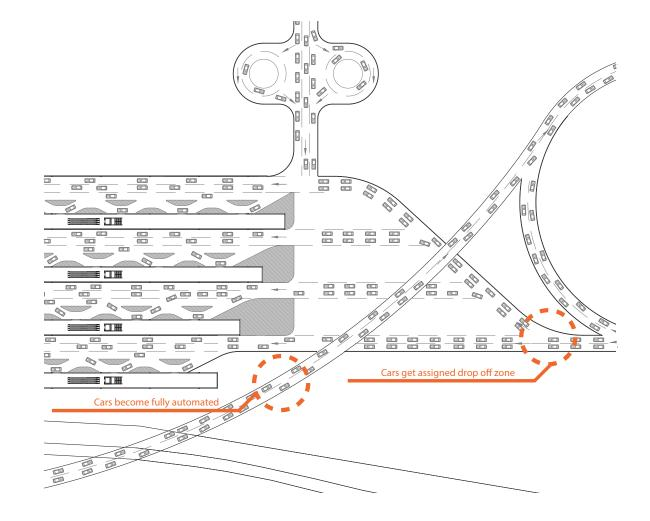
7.13 Control Points. This explains where will the vehicle becomes fully automated and the transit hub will assign a drop off area for the passenger.
