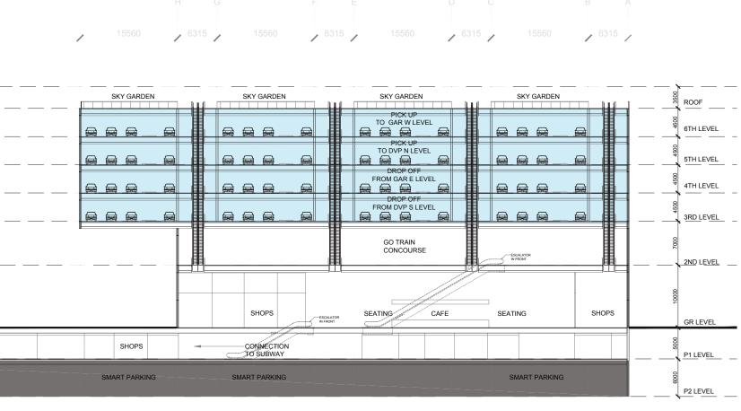
7.3 N-S Section. There are 4 lanes on the drop off/ pick up levels, and the lower levels will be utilized for smart parking.
