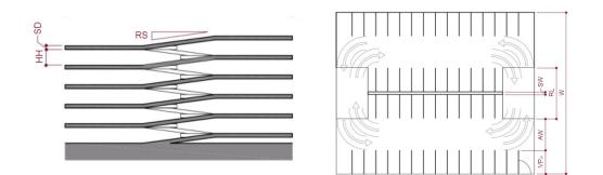
STALL ANGLE STALL DEPTH AISLE WIDTH STRUCTURAL WIDTH STRUCTURAL DEPTH HEAD HEIGHT RAMP SLOPE WIDTH
