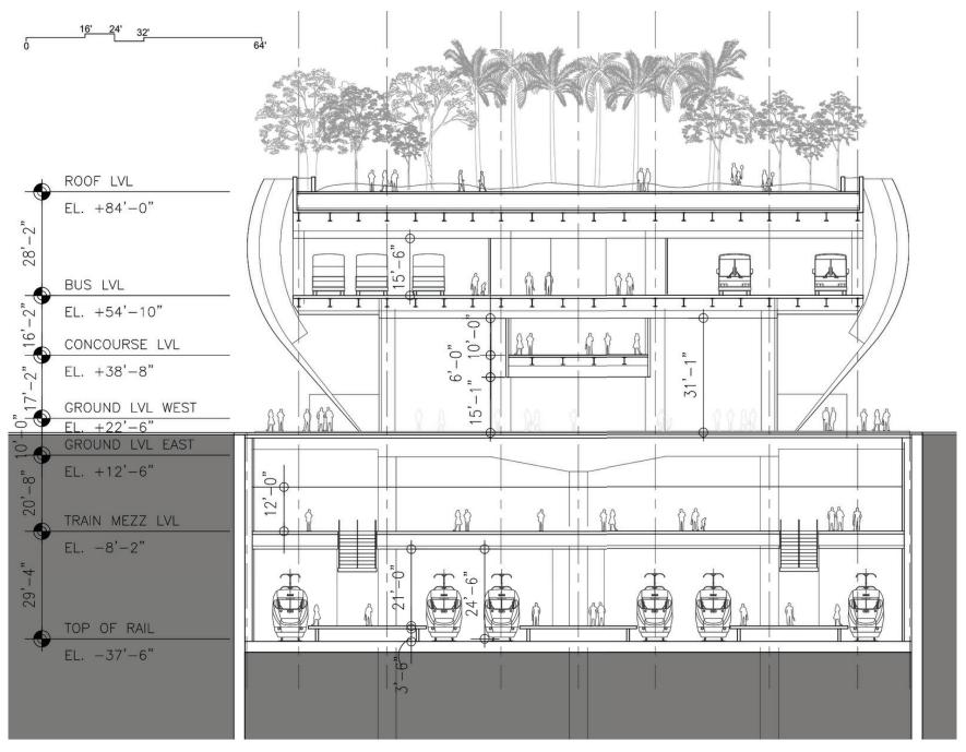
5.4 Transbay Section. This section shows the individual transit system in relation to each level. The lowest level is for trains and the second level is for bus.
