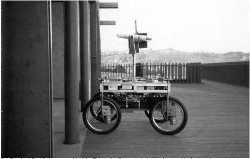
2.1 Stanford Cart Autonomous Vehicle. This is the first invented driverless cart in the bare bones structure.
