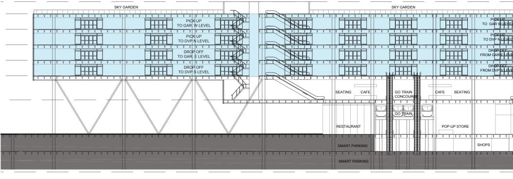
7.2 E-W Section. This section shows the 3rd to 6th floors are dedicated to drop off and pick up from or to the highways, and the passengers will connect to the transit they wish.
