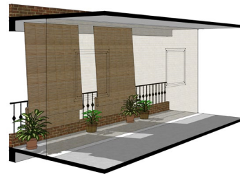
Figure 3.19 Operable Bamboo Chick Blinds
