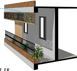
Figure 3.18 Jali/meshwork screen in the corridor to prevent direct sunlight
