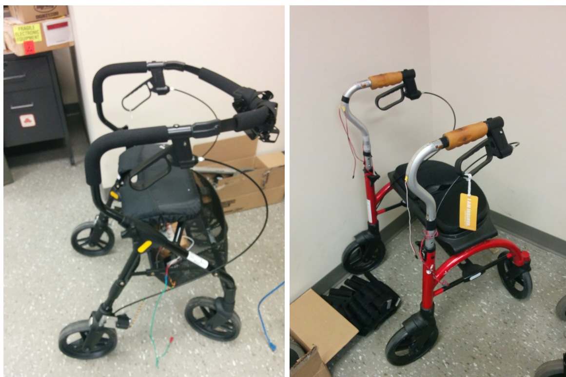
Figure 2.1: Walkers modified with automatic braking(left) and force sensors(Right)
