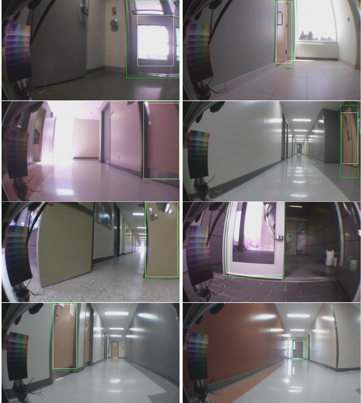
Figure 5.5: Positive Detections in Door YOLO Network. Green boxes indicates ground truth and white boxes are found boxes.
