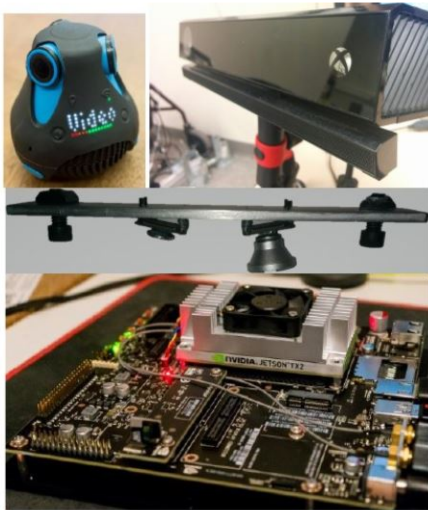
Figure 2.8: Giroptic 360° camera(top left), Kinect (top right),RPi cameras mounted with and without lens(middle), jetson tx2 with camera.(bottom)
