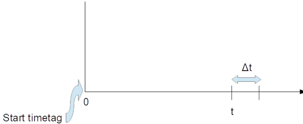
Figure 5.3: Following an arbitrary detector click (also called the start time tag), we consider a time interval of width \Delta t after time t has elapsed since the start time tag.
