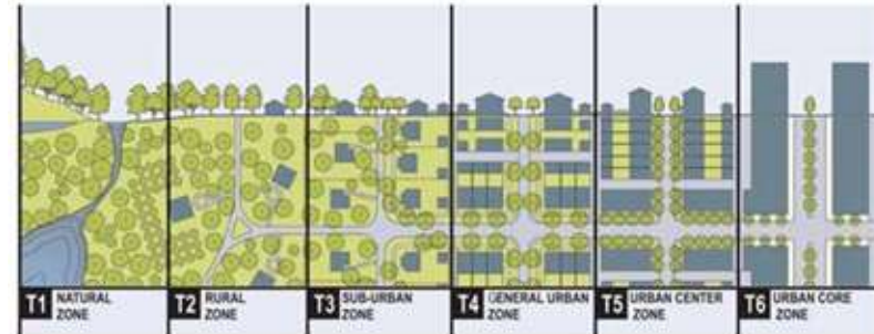
Figure 4.8 Top: Urban Transect with six rural to urban zones. Andres Duany, Jeff Speck, Kike Lydon, The Smart Growth Manual , McGraw Hill (2009) Pg. 1.4
