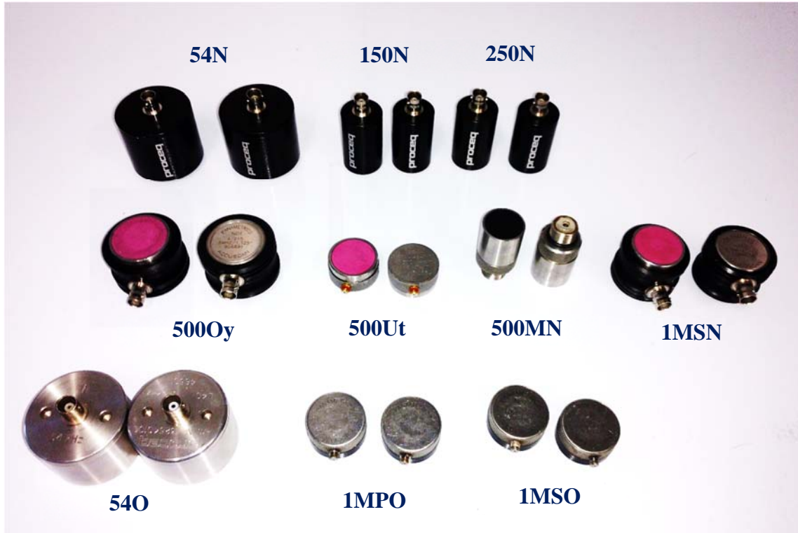
Figure 3-1: Types of the characterized ultrasonic transducers.
