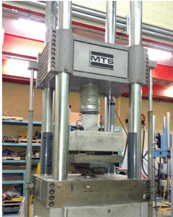
Figure 7-6. The main frame of the compression machine MT35000KN for testing concrete models.
