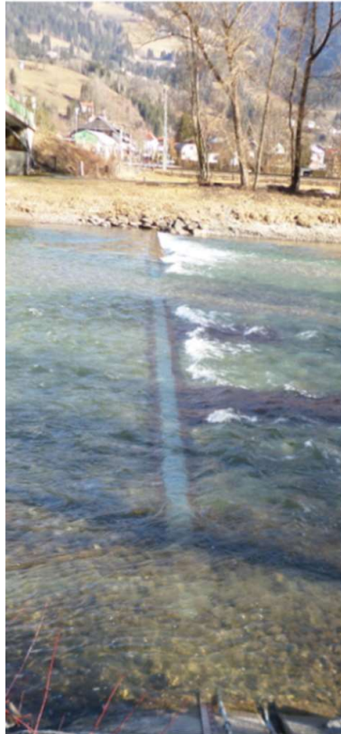
Figure 12: Geophone installation across a channel (Habersack, et al., 2016)
