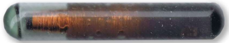
Figure 17: 12mm Passive Integrated Transponder Tag. Taken from Oregon RFID (June 3rd, 2018)
