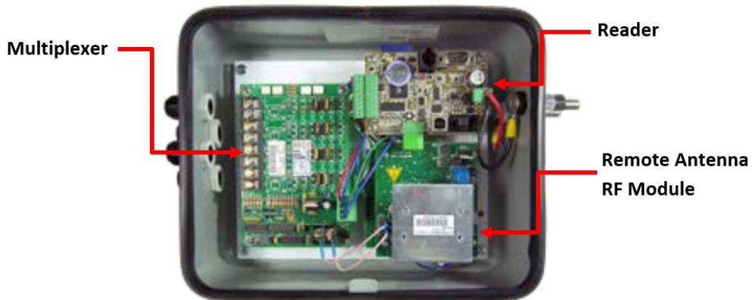
Figure 42: Oregon RFID Multi-antenna Reader (Oregon RFID, 2018)
