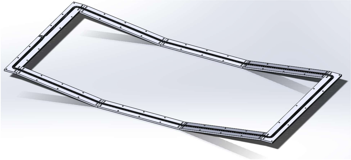
Figure 49: Assembly of antenna casing. Side pieces and end pieces are 75cm and 100cm long respectively
