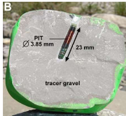
Figure 21: Example of the insertion method for RFID tags. (Leibault et al., 2012)
