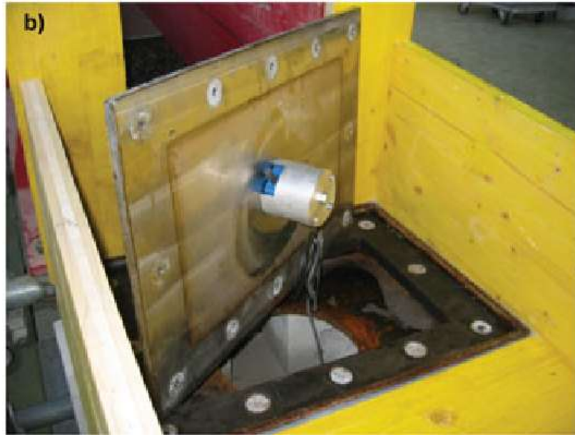
Figure 11: Geophone placed in the Erlenbach stream (Rickenmann et al., 2012)
