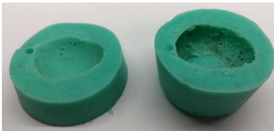
Figure 38: Silicon mold used to create the synthetic stone
