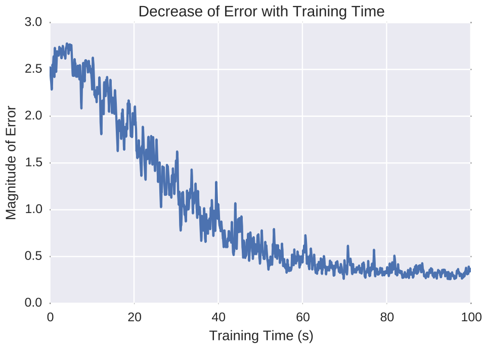
FIGURE 3.7: Error magnitude in the Fast-Net decreasing with training received from the Slow-Net feedback of each trial.
