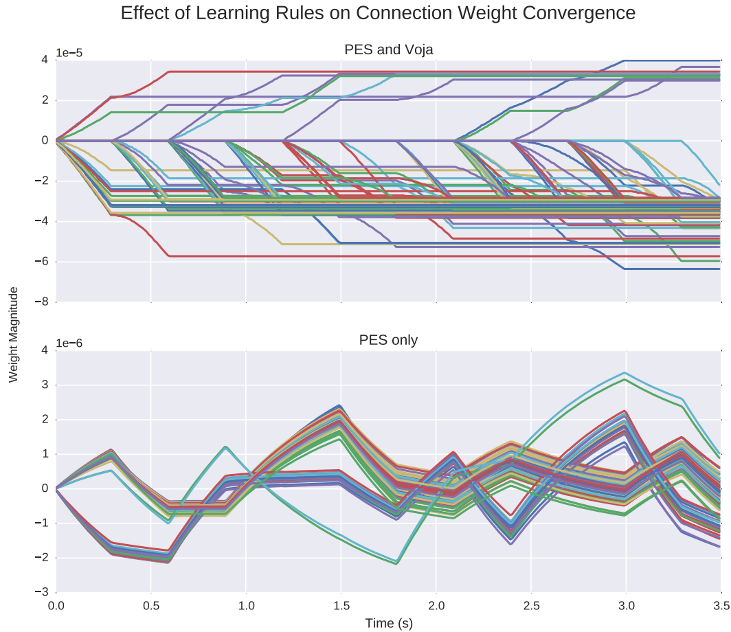
FIGURE 3.6: Fast-Net decoder weights changing over time while being simulated separately from Slow-Net and learning the sum transformation given inputs of two addends concatenated. Ensemble decoders learned using only the PES rule never converge. However, if learned using Voja with PES, ensemble decoders quickly settle to a stable value.
