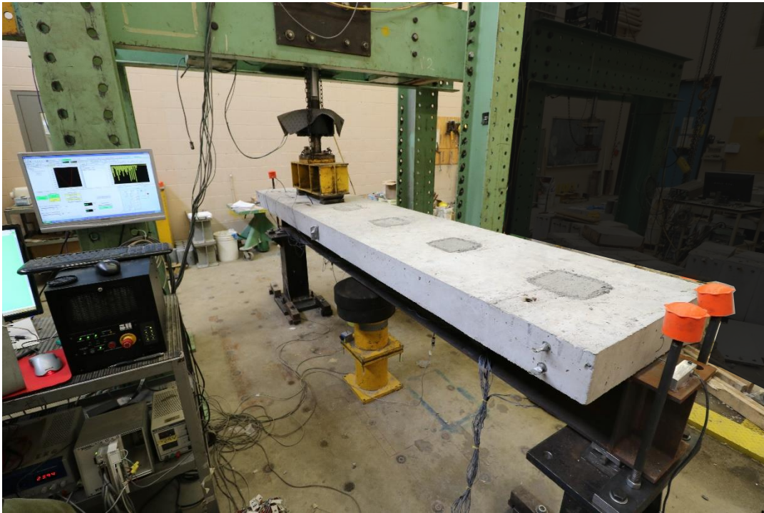
Figure 3-2. PS specimen during fatigue testing.
