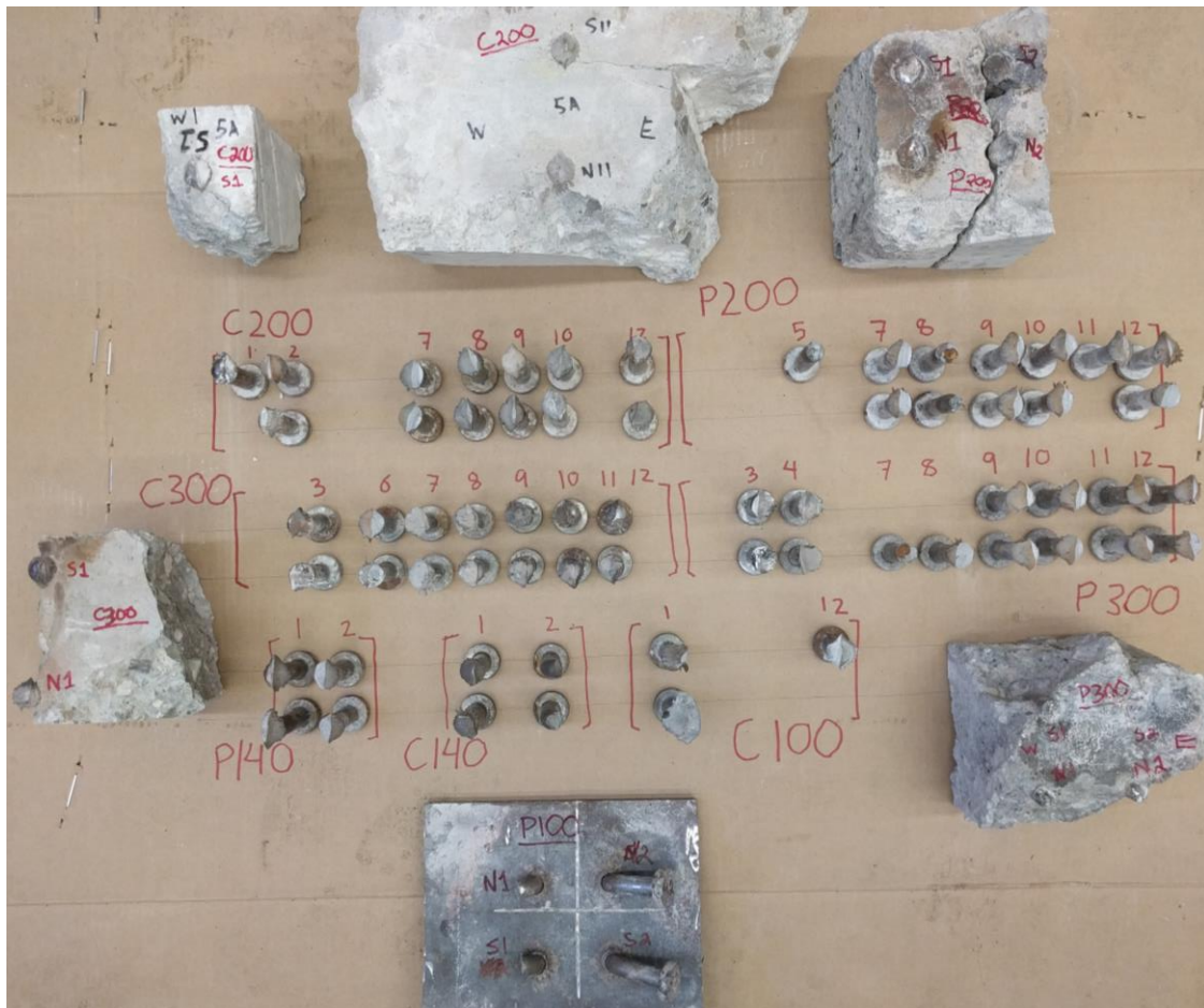
Figure 4-19: Overview of all studs that failed in fatigue.
