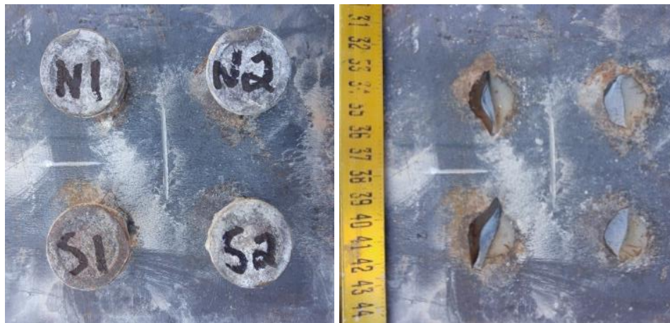
Figure 4-15: Critical stud group of specimen PS140 before (left) and after (right) bend test.
