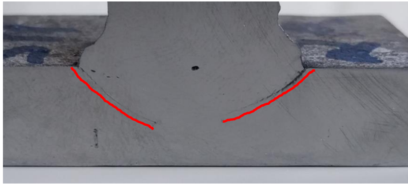
Figure 4-18: Cross-section of a failed stud connector (fatigue cracks highlighted).
