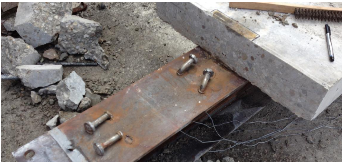
Figure 4-12: Autopsy on CS140, showing N1/S1 failed bend tests and N2/S2 passed bend tests.
