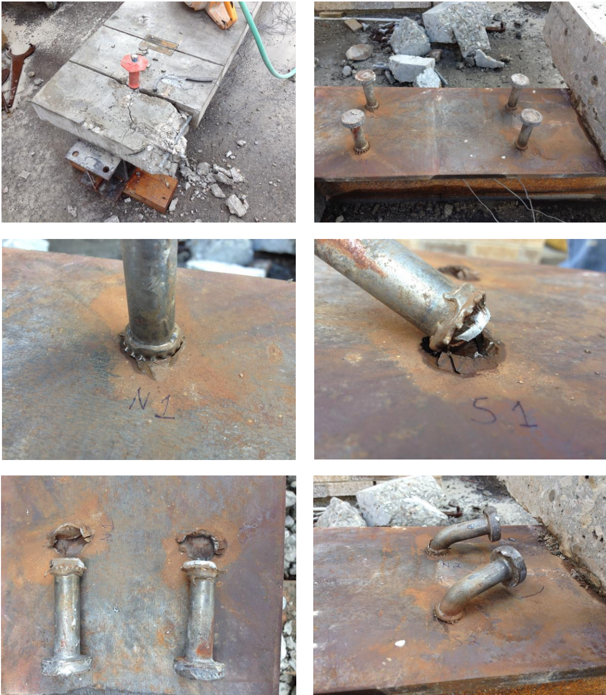
Figure 4-13: Autopsy procedure in image form featuring N1/S1 and N2/S2 of CS140.
