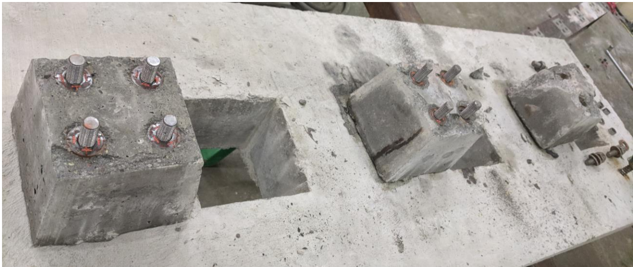
Figure 4-14: Autopsy procedure in image form featuring N1/S1 and N2/S2 of CS140.
