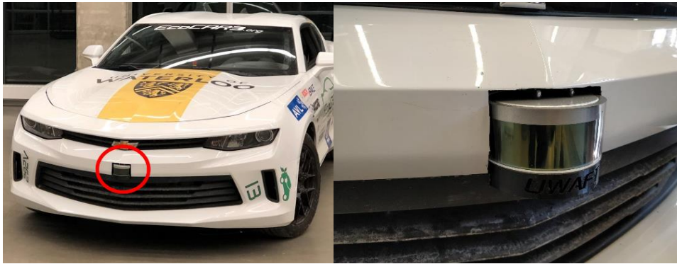
Figure 17: UWAFT PHEV Velodyne LiDAR Integration
