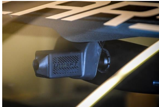
Figure 16: UWAFT PHEV OmniVision Camera Integration
