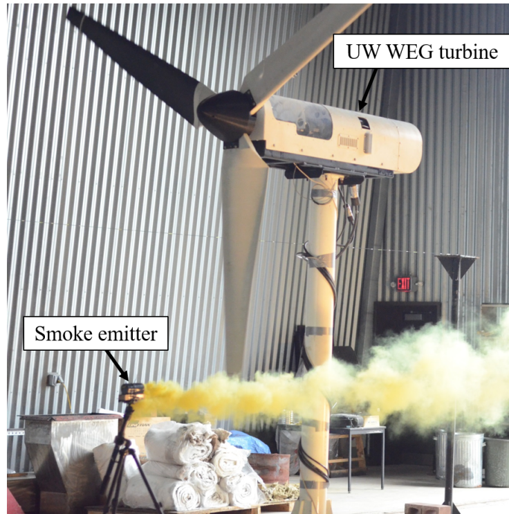
Figure 4.7: Single colour smoke visualization experiment setup
