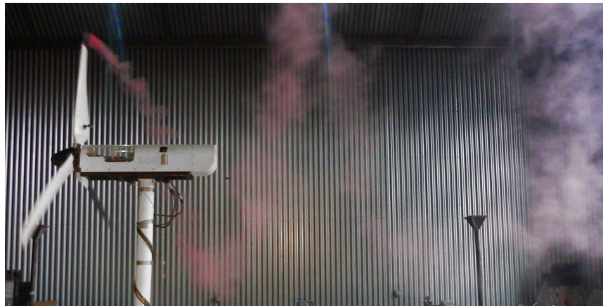
Figure C.3: Blade tip smoke visualization of the UW WEG turbine for \lambda = 1.7
