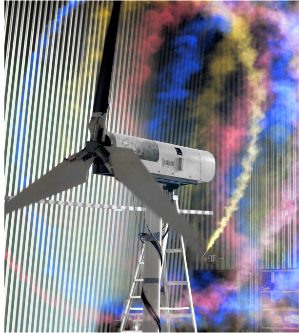
Figure 5.8: Crosswise view of the blade ignited smoke visualization of the UW WEG turbine for \lambda = 4.3 and \gamma = 0^\circ
