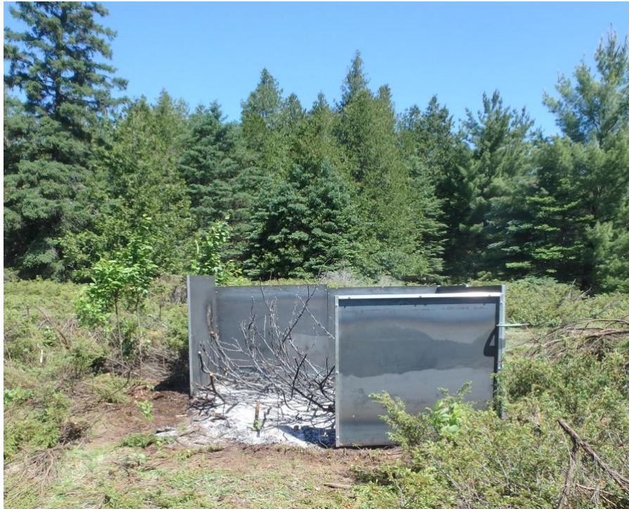
Figure 3. An assembled burn box with two panels removed to show interior of the burn area. Perimeter of the box has a 1 m vegetation buffer to prevent ignition of non-target vegetation.
