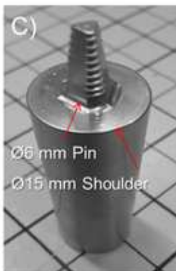
10° tapered, M6 threaded three flats H13 steel tool
