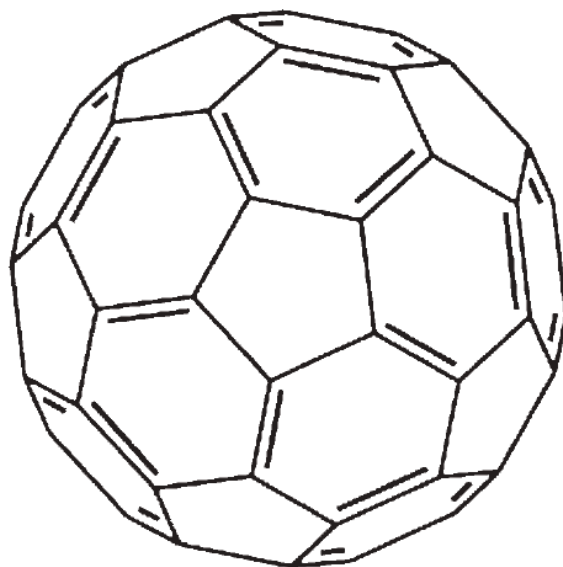
Figure 2.1. A molecular structure of buckminsterfullerene, C 60 . [5] Reprinted with permission from Elsevier
