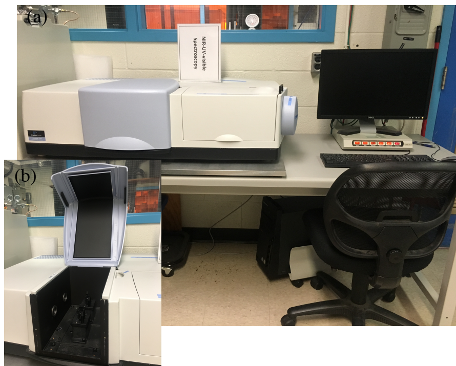
Figure 3.2. (a) The UV-Vis spectrometer located at WATLab room 080 in the chemistry 2 building. (b) The holders chamber for the sample and reference cuvettes.
