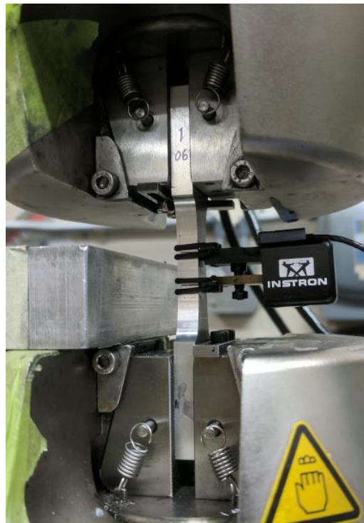
Figure 12 Fatigue testing of smooth specimen on the Instron 8874 machine with strain measurement by extensometer. A block of aluminium was placed beside the specimen as a physical safeguard against accidental crushing of the extensometer.
