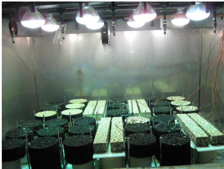
Figure 2-16 Inside view of APWS showing mixture sample under conditioning [35]
