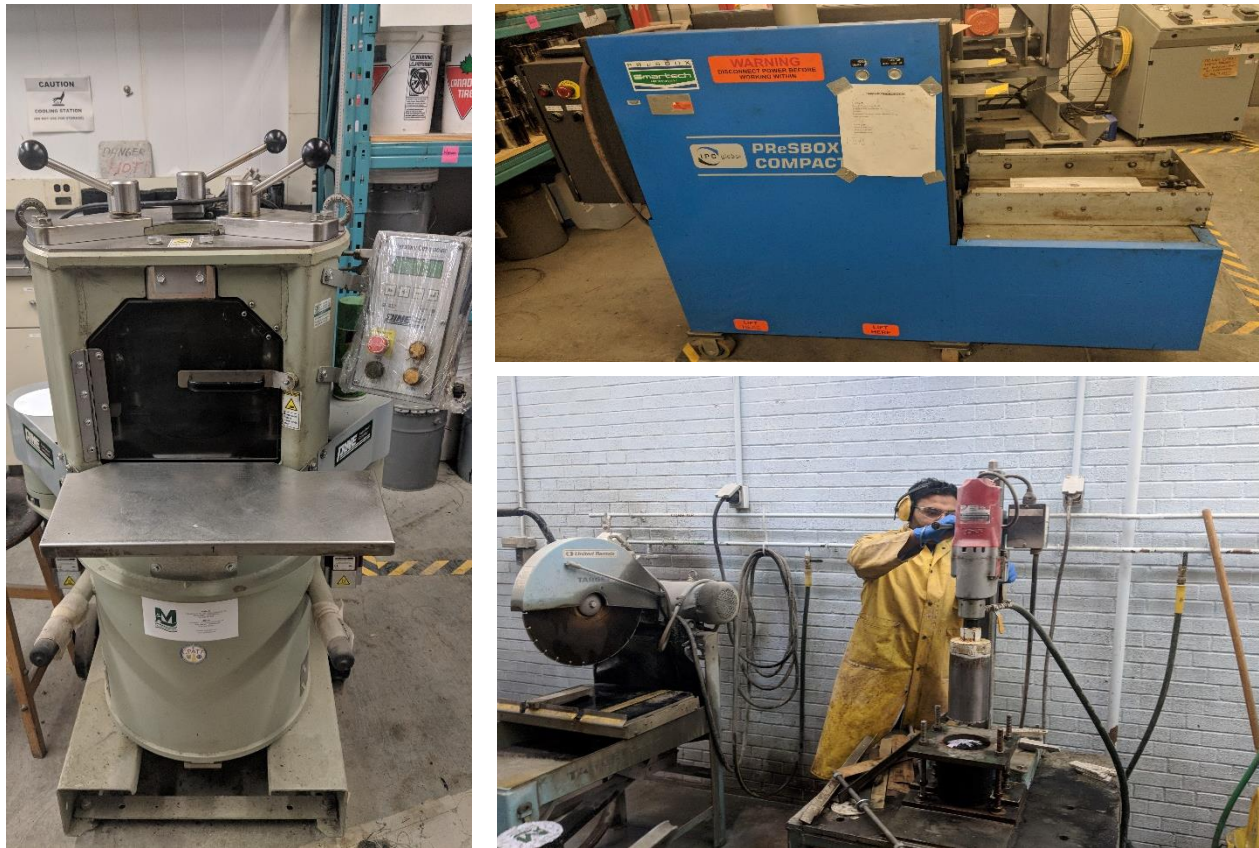
Figure 3-3 Compaction, Cutting & Coring at CPATT Laboratory
