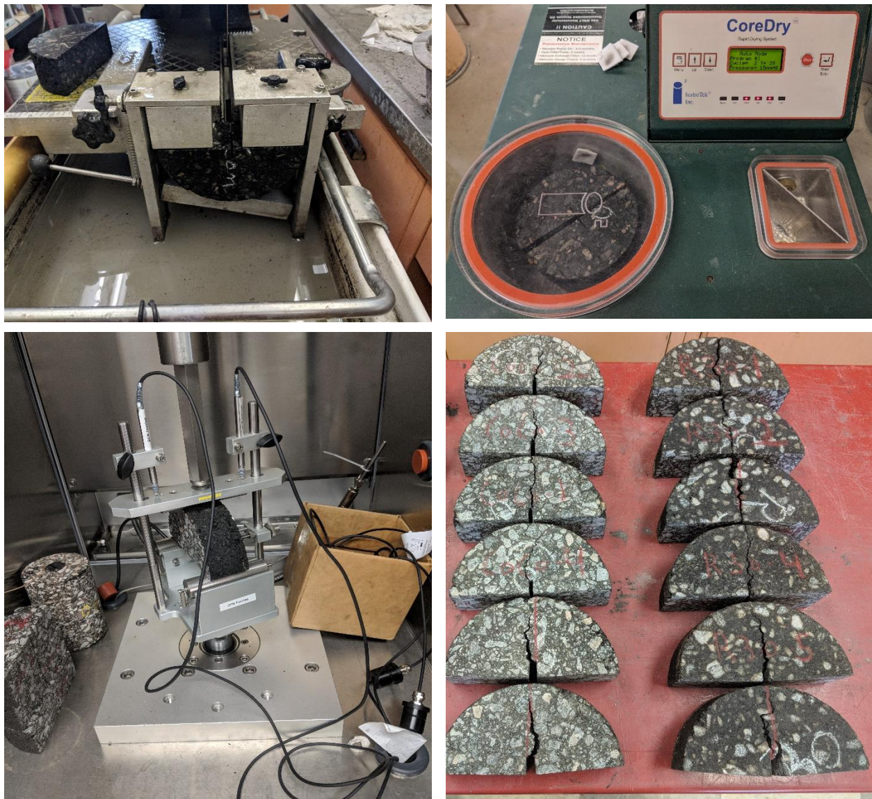
Figure 3-11 Different Stages of SCB Test (Cutting & Notch Preparation, Drying followed by Temperature Conditioning, Testing using DTS-30 Frame, and Samples after Testing)
