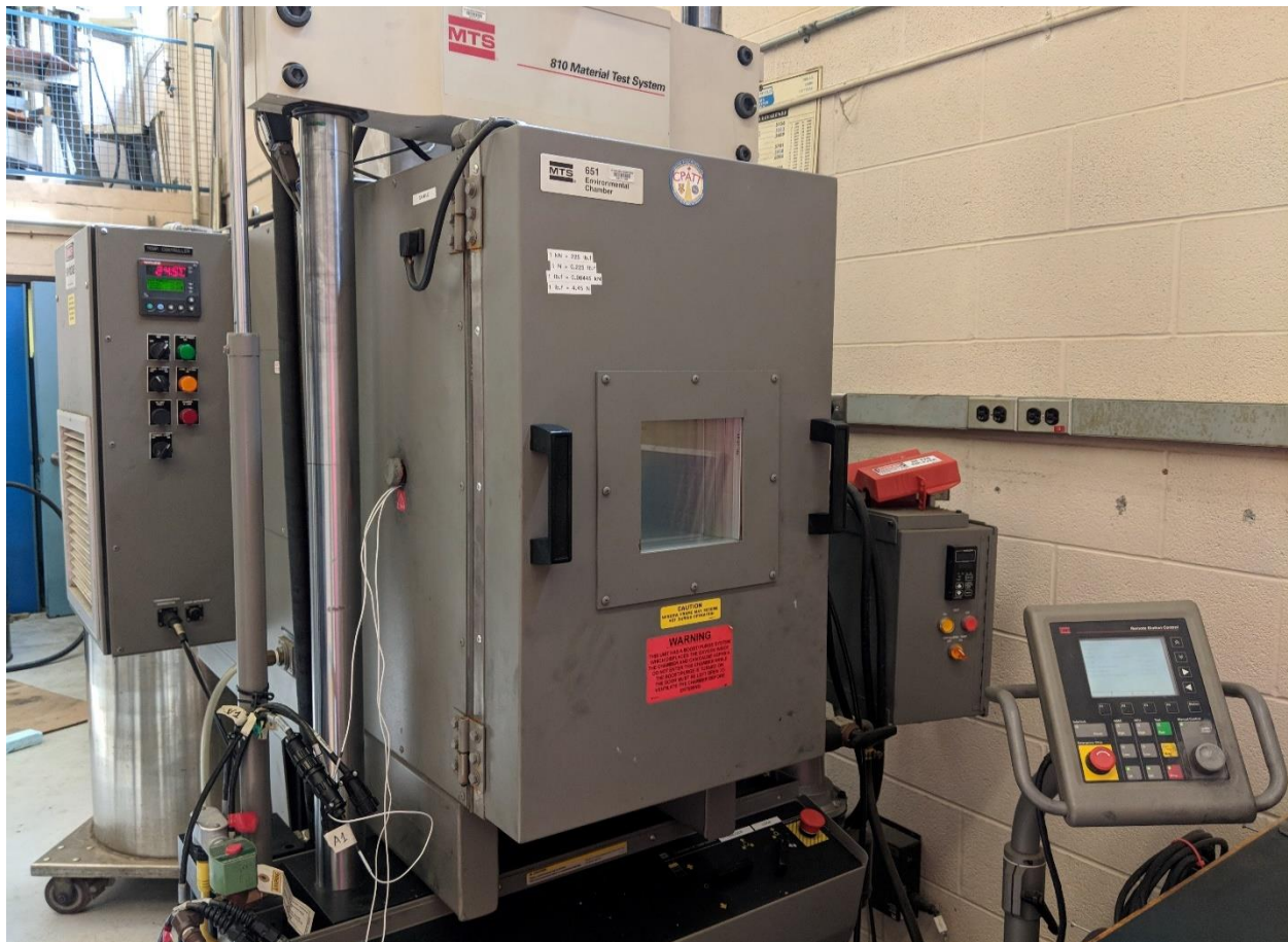
Figure 3-10 810 MTS Loading Frame and 651 MTS Environmental Chamber
