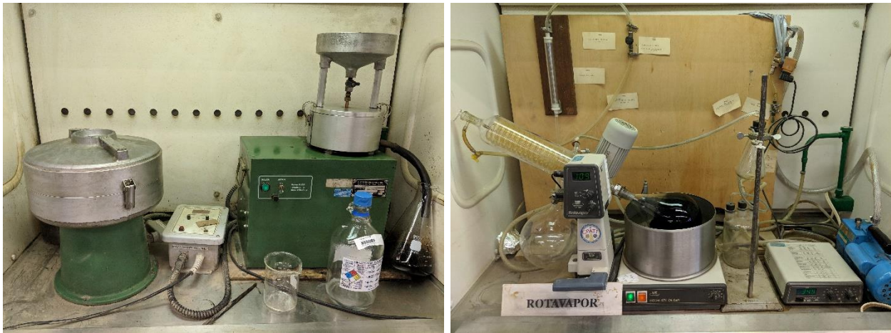
Figure 3-7 Centrifuge Extractor, High-Speed Centrifuge and Rotavapor at CPATT lab
