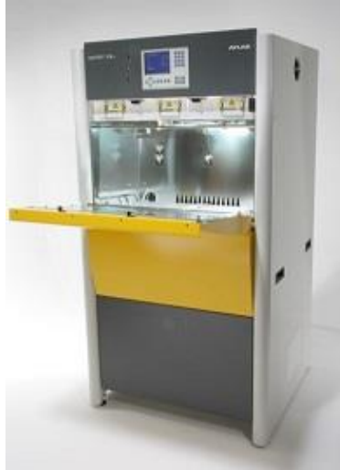
Figure 2-15 Atlas Weatherometer Suntest XXL [33]
