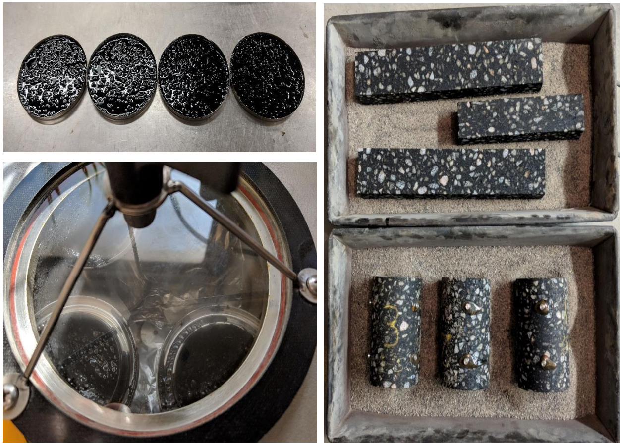
Figure 3-4 PAV residue, Degassing & AASHTO R30-02 Compacted Sample Conditioning
