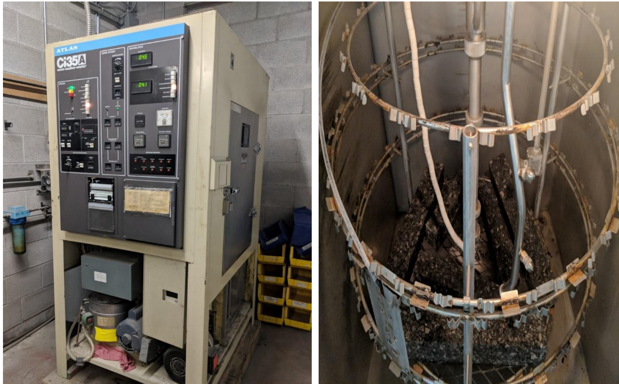
Figure 3-5 Atlas Weatherometer Ci35A showing external, and internal view with metal mesh platform for beam support
