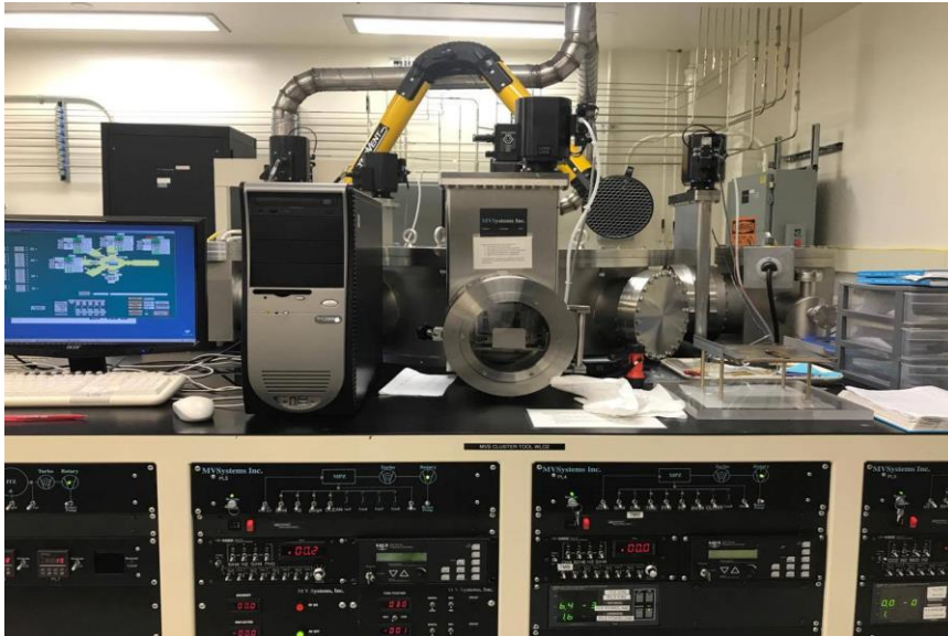
Figure 2.5 Multi-chamber PECVD Cluster System.
