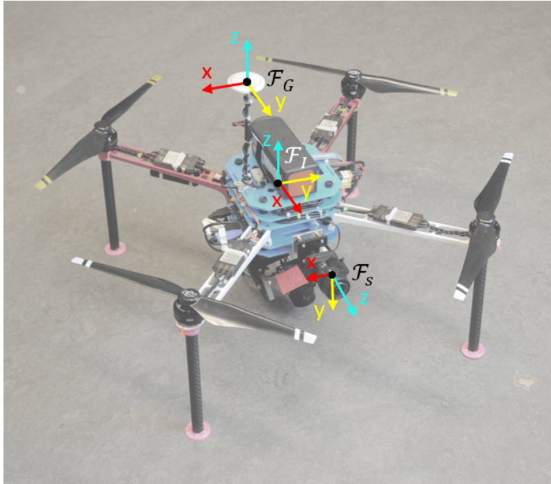
Figure 4.2: Custom MAV hardware with 2-DOF gimbal based DCC mounted on bottom. Frames \mathcal{F}_s , \mathcal{F}_I , \mathcal{F}_G denote the static camera, IMU, and GPS frames, respectively.
