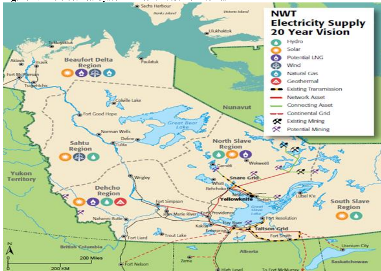
Figure 2: The electrical system in Northwest Territories
