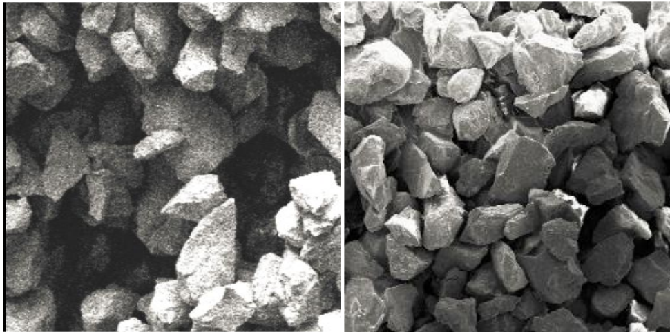
Figure 2.10 Microphotographs showing aggregates and macropores structure, and regular single-grained packing structure (Benahmed et al., 2015)
