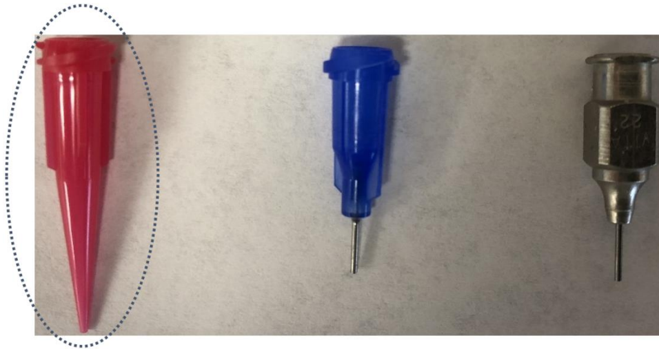
Figure 26. Different nozzle shapes with various materials such as plastic, plastic-metal, and metal.
