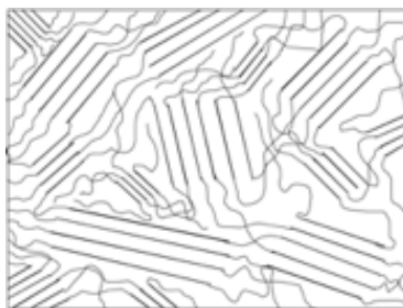
Figure 3.2: Fringed micelle model of polymer crystal structure. Figure source: “Principles of polymer chemistry” by Paul J. Flory, Cornell University Press , 1953 [23].
