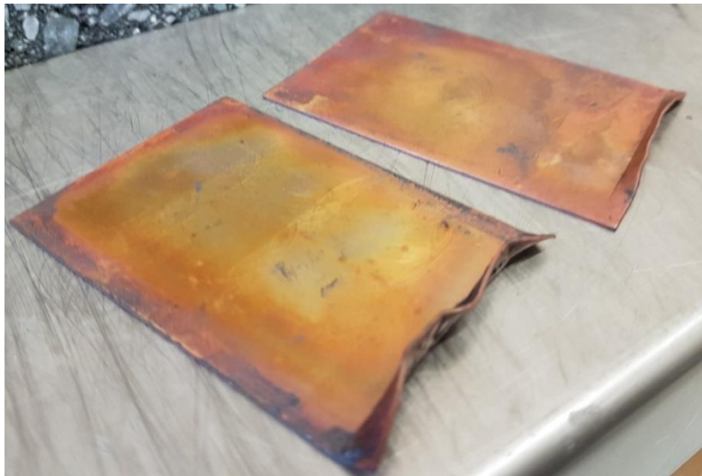
Figure 6.10: Damaged Copper Sleeves after Testing
