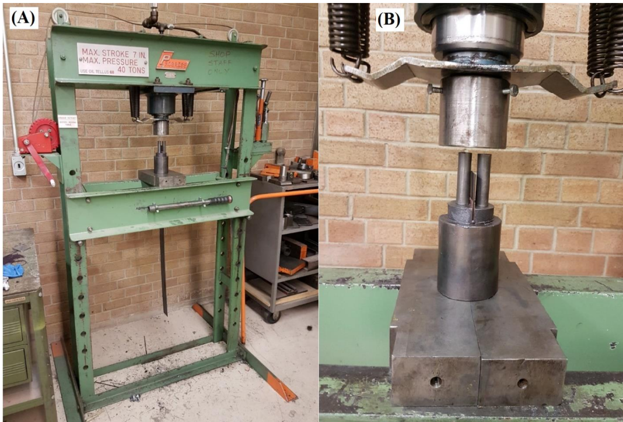
Figure 6.6: (A) Presetting Rig Apparatus (B) Setup of the Anchorage in the Presetting Rig Apparatus
