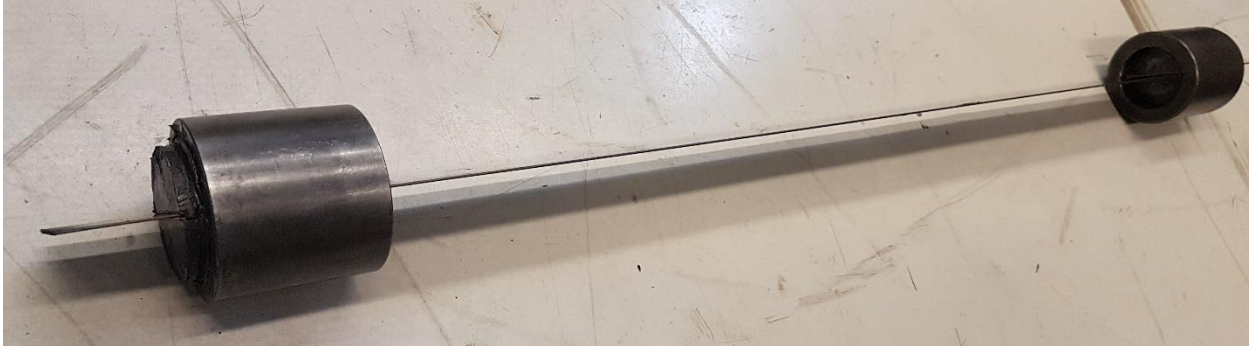
Figure 6.5: Assembled Wedge Anchorages and CFRP Plate
