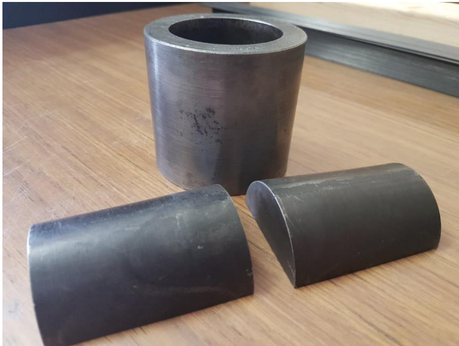
Figure 6.3: Optimized Wedge Anchorage
