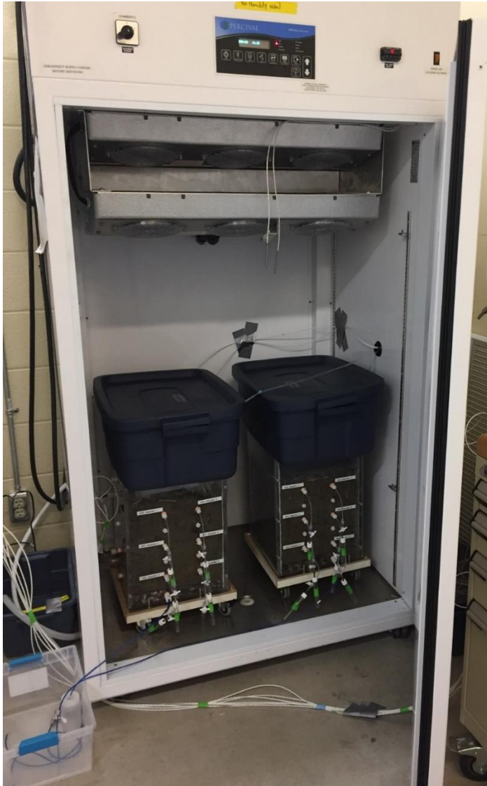
Supplementary Figure A1 Photograph of experiment set up including soil monoliths inside temperature controlled chamber.
