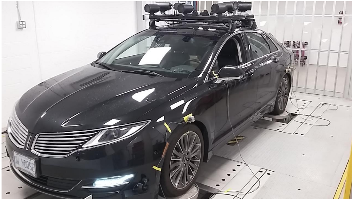
Figure 2.9: Lincoln MKZ on 4-post test rig
