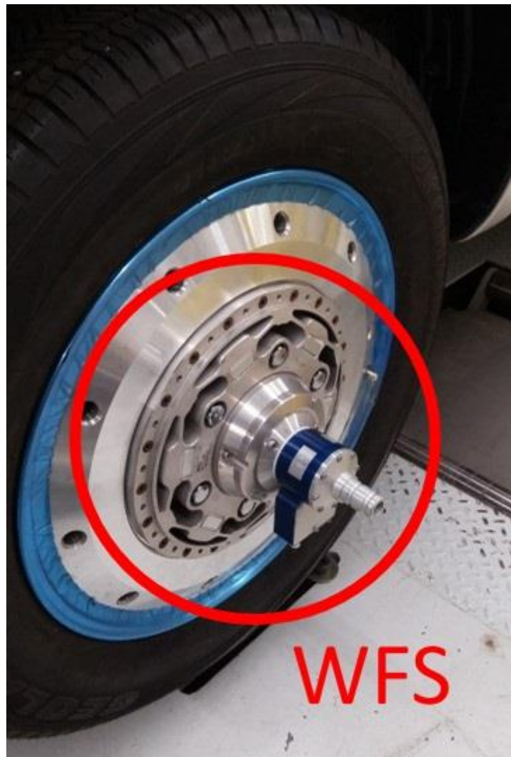
Figure 2.2: Wheel Force Sensor (WFS) attached to custom wheel rim
