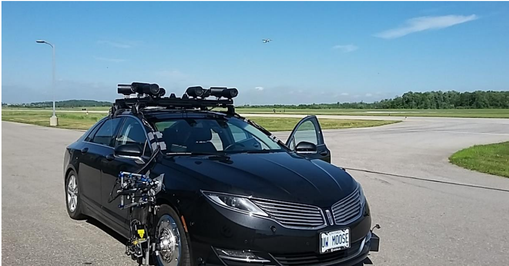
Figure 2.8: Lincoln MKZ at Waterloo International Airport for drag testing
