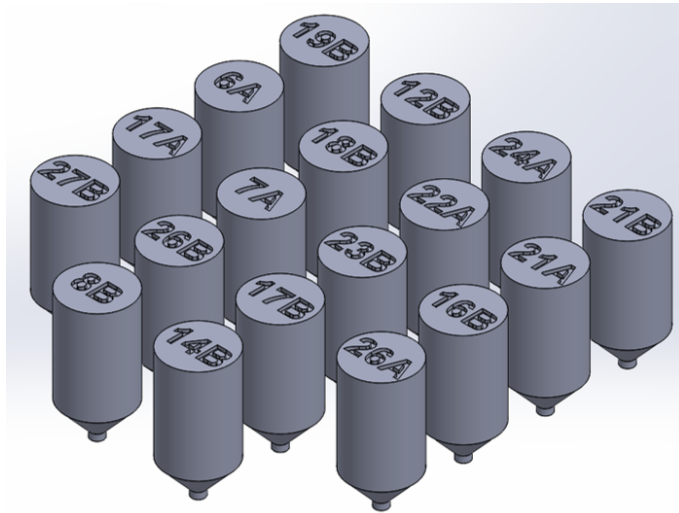
Figure 3.3: The input CAD file showing the random distribution of the samples on the first printing batch build plate.
